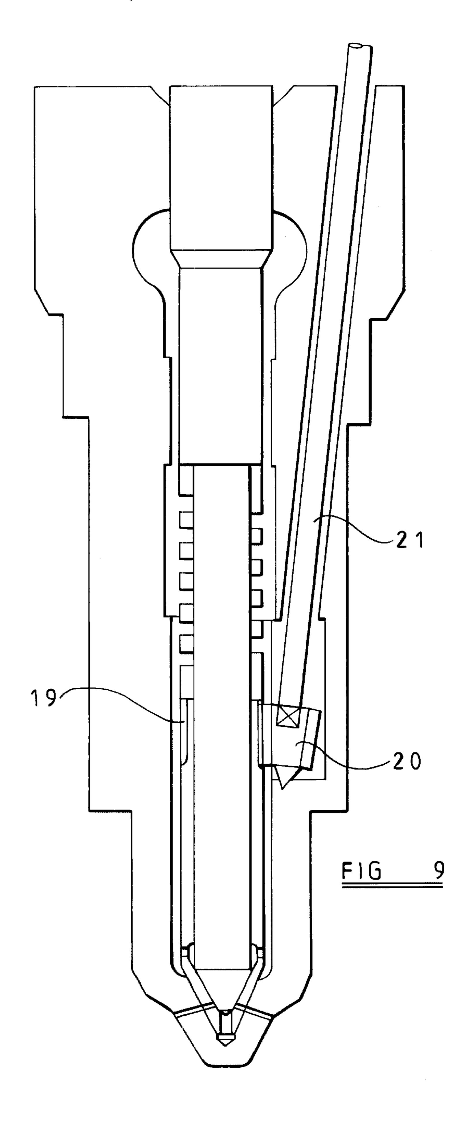
This invention relates to a fuel injector, and in particular to a fuel injector suitable for use in delivering fuel under pressure to a cylinder of a compression ignition internal combustion engine.
