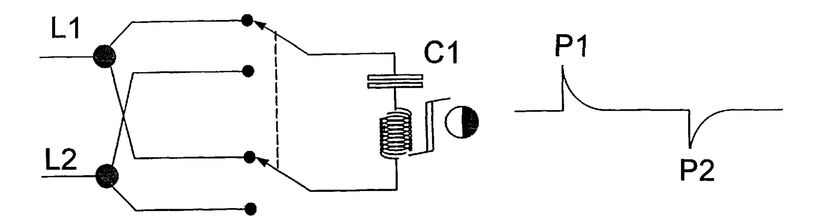
Figure 1 Current pulse to magnetic latch indicator
