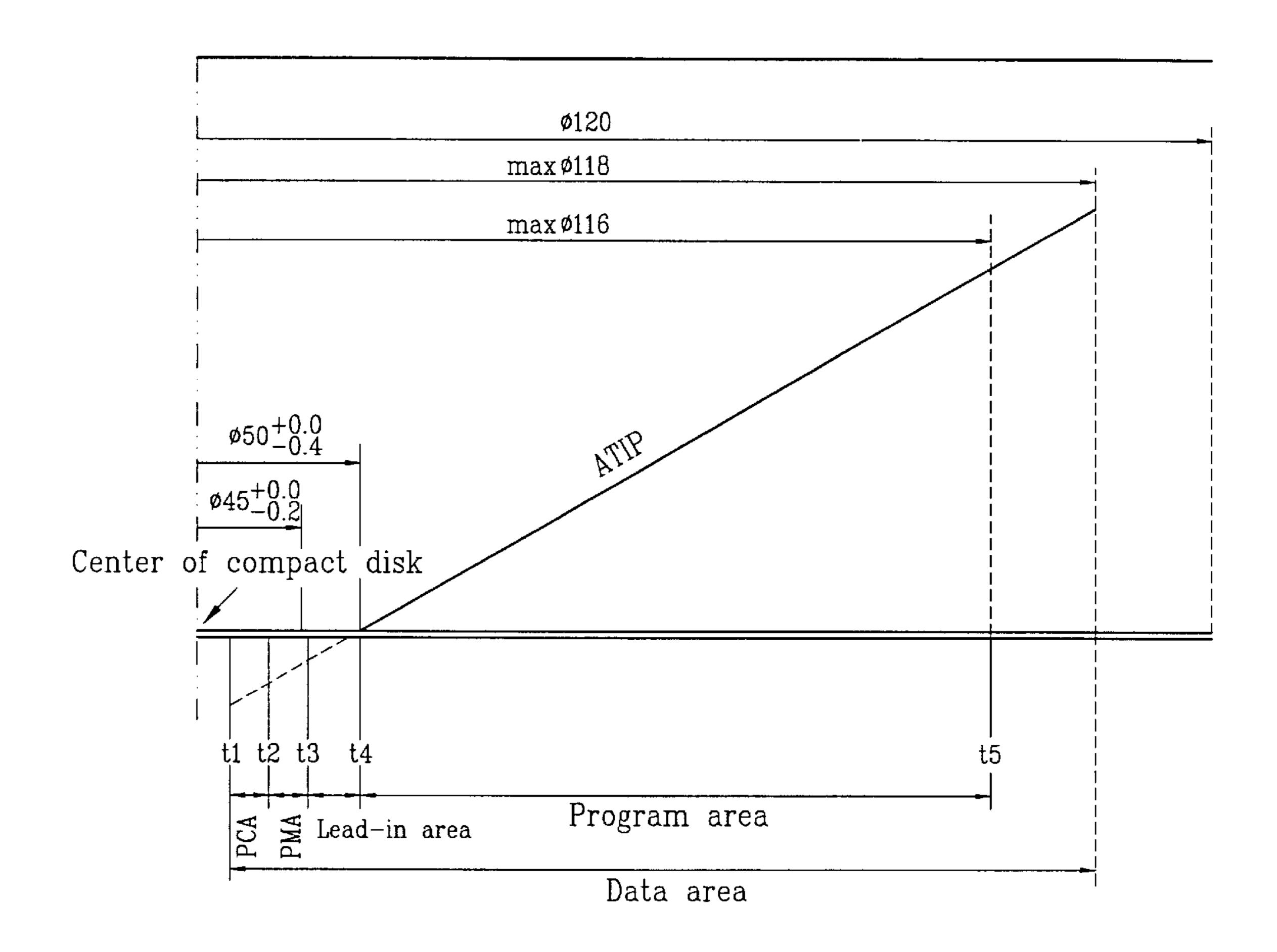
t1 = Start time PCA = t3 - 00:35:65 t2 = Start time PMA = t3 - 00:13:25 t3 = Start time Lead-in Area = encoded in ATIP t4 = End time Lead-in Area = 99:59:74 Start Time Program Area = 00:00:00 t5 = Last possible start time = encoded in ATIP of Lead-out Area
