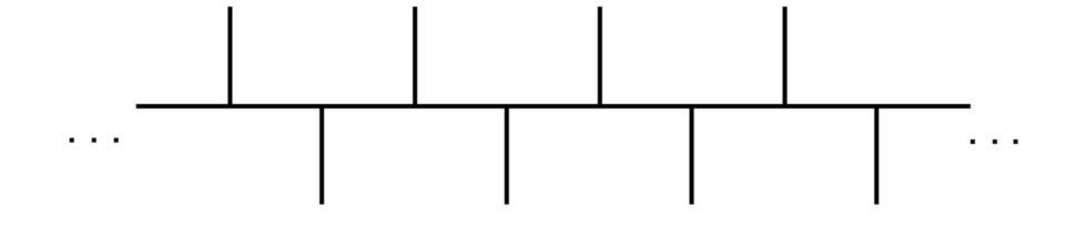
The methyl groups attached to the tertiary carbon atoms of successive monomeric units in the chain lie on alternate sides of the plane of the polymer.
