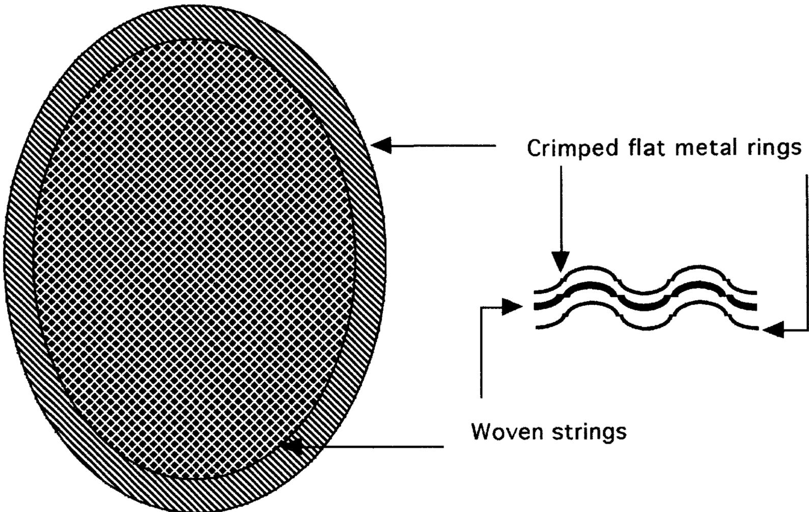
**Crimped flat metal rings**
