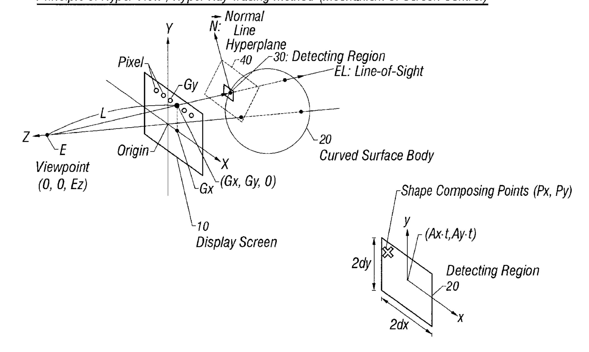
Ray Tracing Method (Mechanism of Screen Conti FIG. 1 (1)
