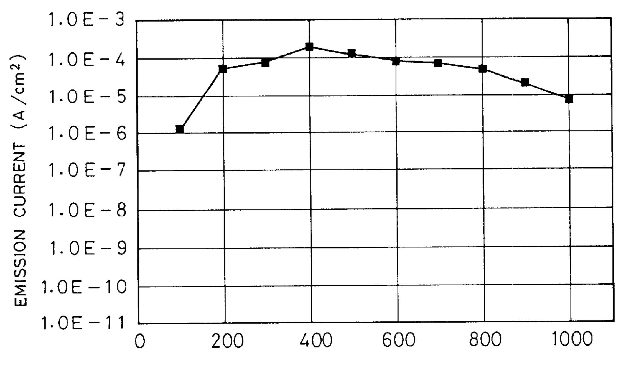
THICKNESS OF INSULATOR LAYER (nm)
