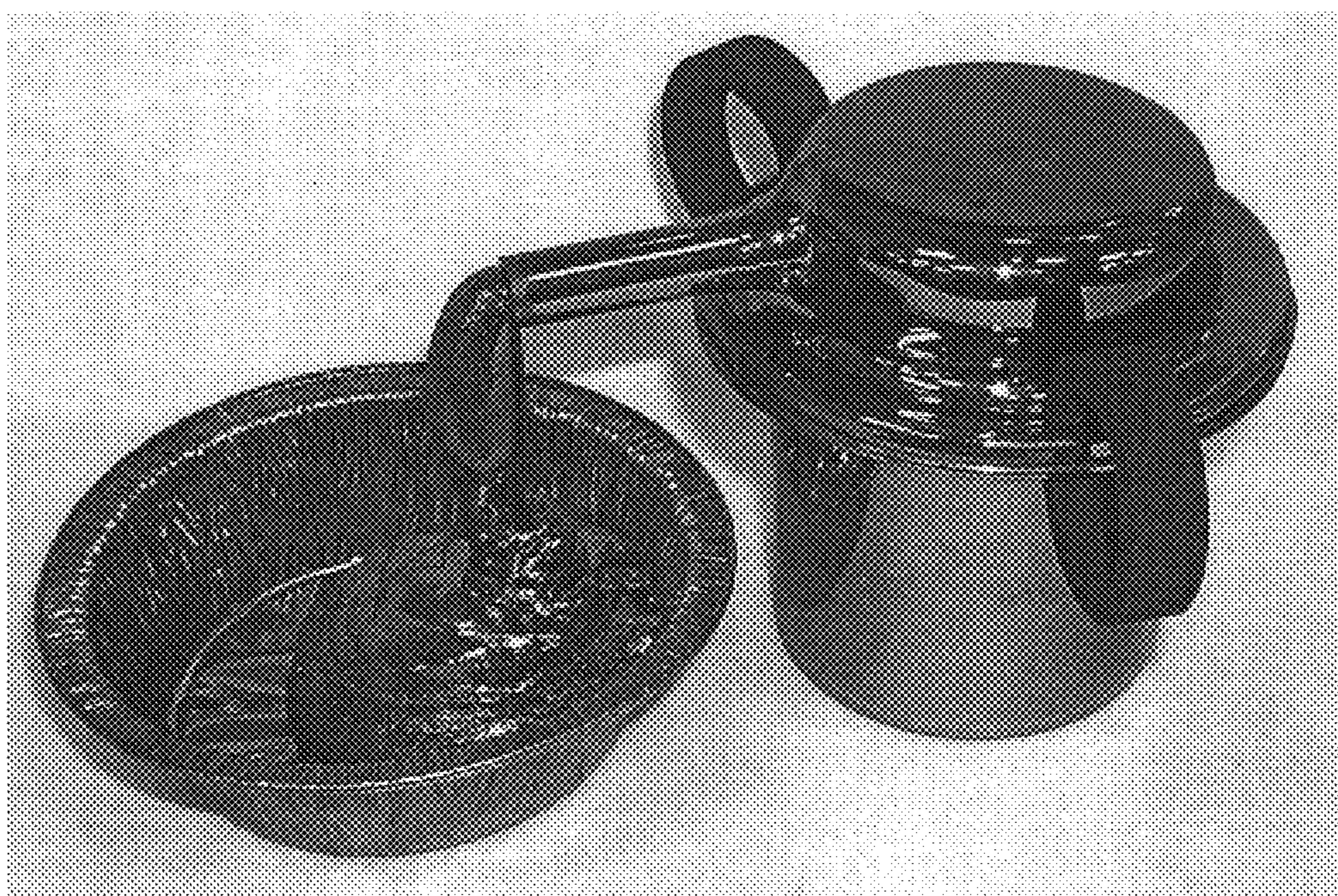
Figure 3. Foaming vessel and casting of foam after removing from furnace
