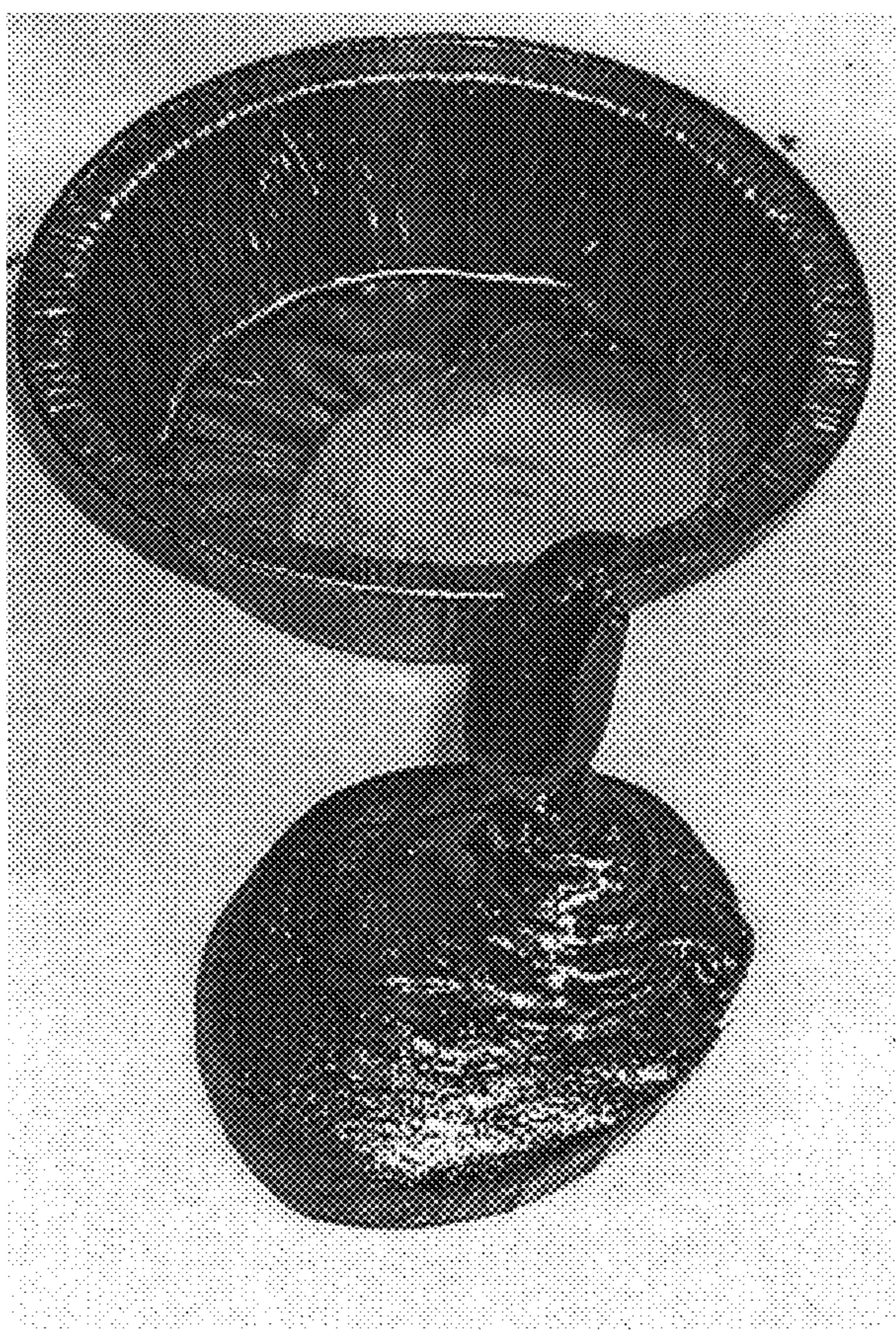
Figure 4. Casting of foam removed from receiving Mold
