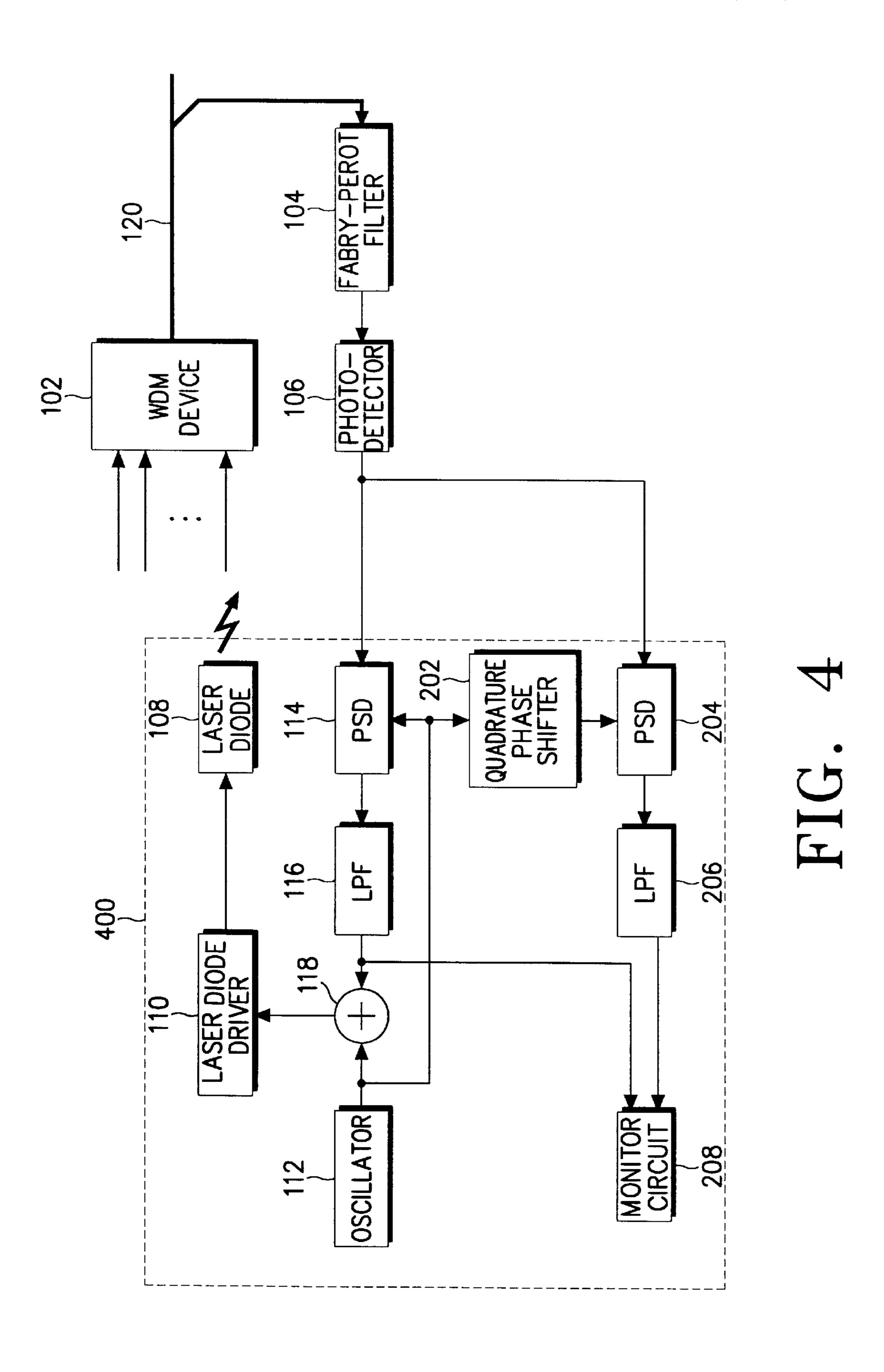
MONITORING THE STABILITY OF THE WAVELENGTH OF A LIGHT SIGNAL IN AN OPTICAL COMMUNICATIONS SYSTEM EMPLOYING WAVELENGTH DIVISION MULTIPLEXING AND HAVING A WAVELENGTH STABILIZATION CIRCUIT
