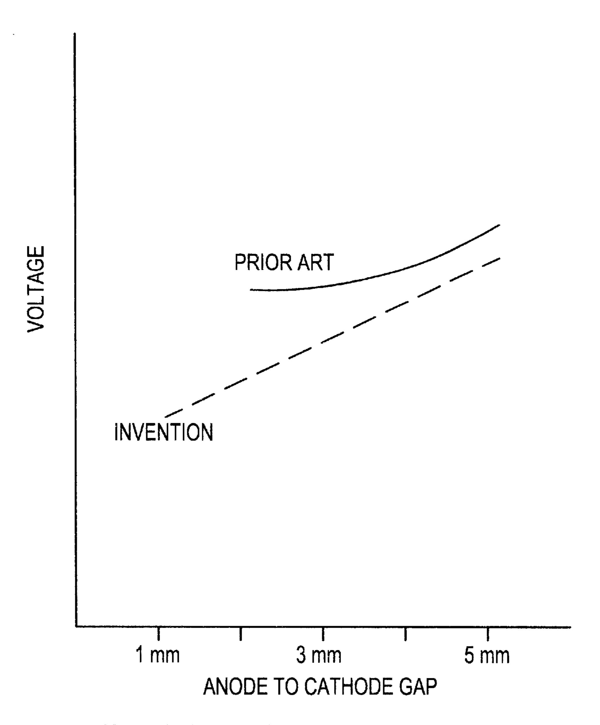
PRIOR ART: 2mm THICK DIAPHRAGM ON CATHODE INVENTION: COMPRESSED DIAPHRAGM FILLS THE GAP DIAPHRAGM THICKNESS REDUCED 1mm BY COMPRESSION
