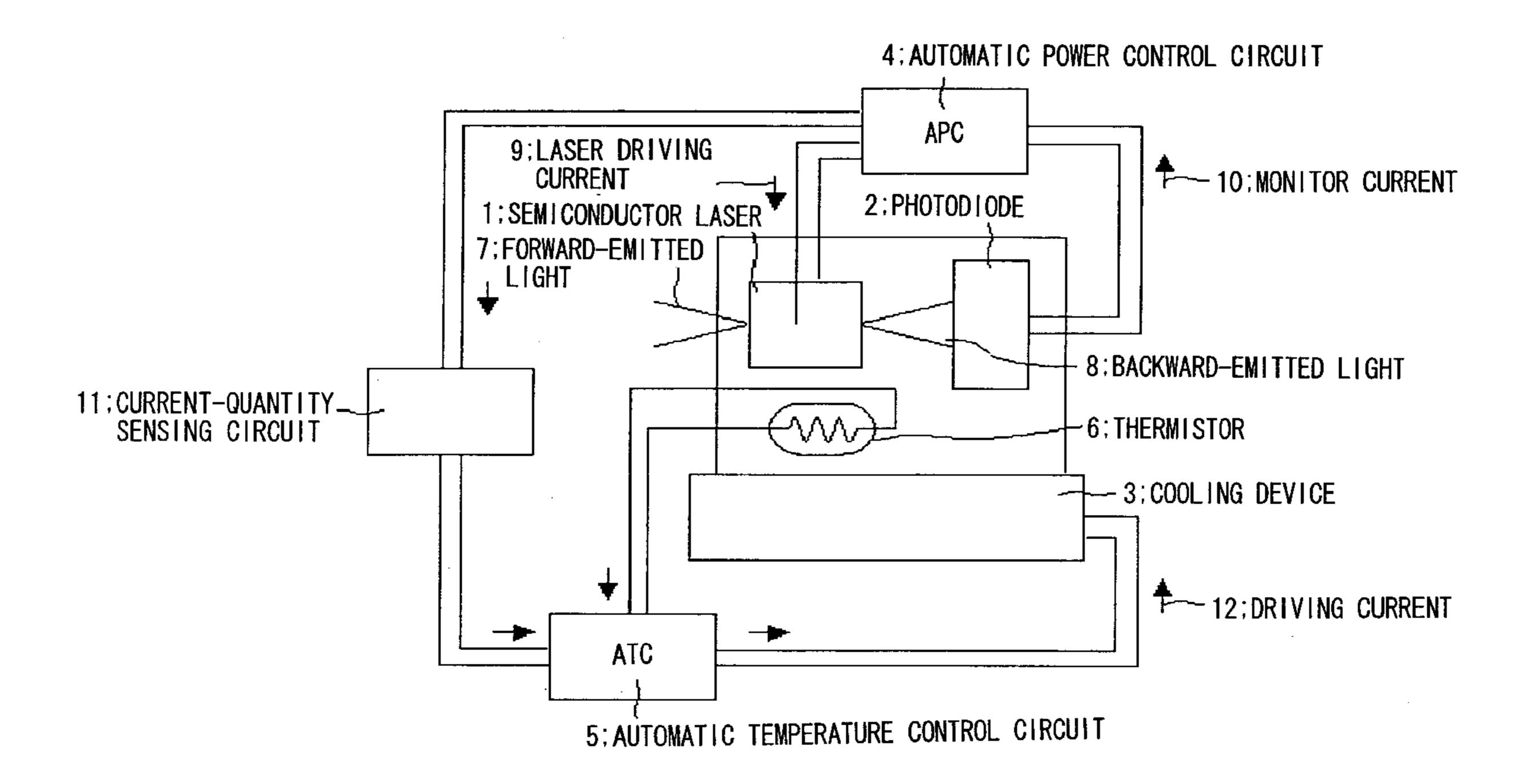
12: DRIVING 8:BACKWARD-EMITTED 10; MON! 6; THERMISTOR 4: AUTOMATIC POWER CONTROI 3; COOL 2:PHOTODIODE CONTROL APC C TEMPERATURE 5; AUTOMATI 9:LASER DRIVING CURRENT : SEM I CONDUCTOR 7: FORWARD-EMITI 1 LIGHT
