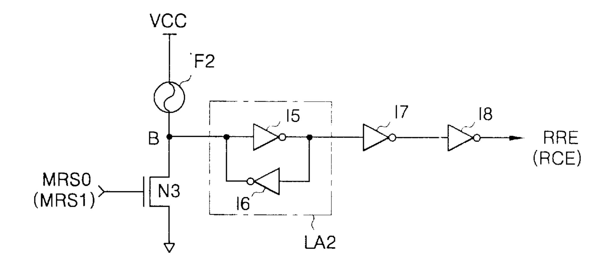
COLUMN REDUNDANT FUSE PROGRAM CIRCUIT COLUMN REDUNDANT
