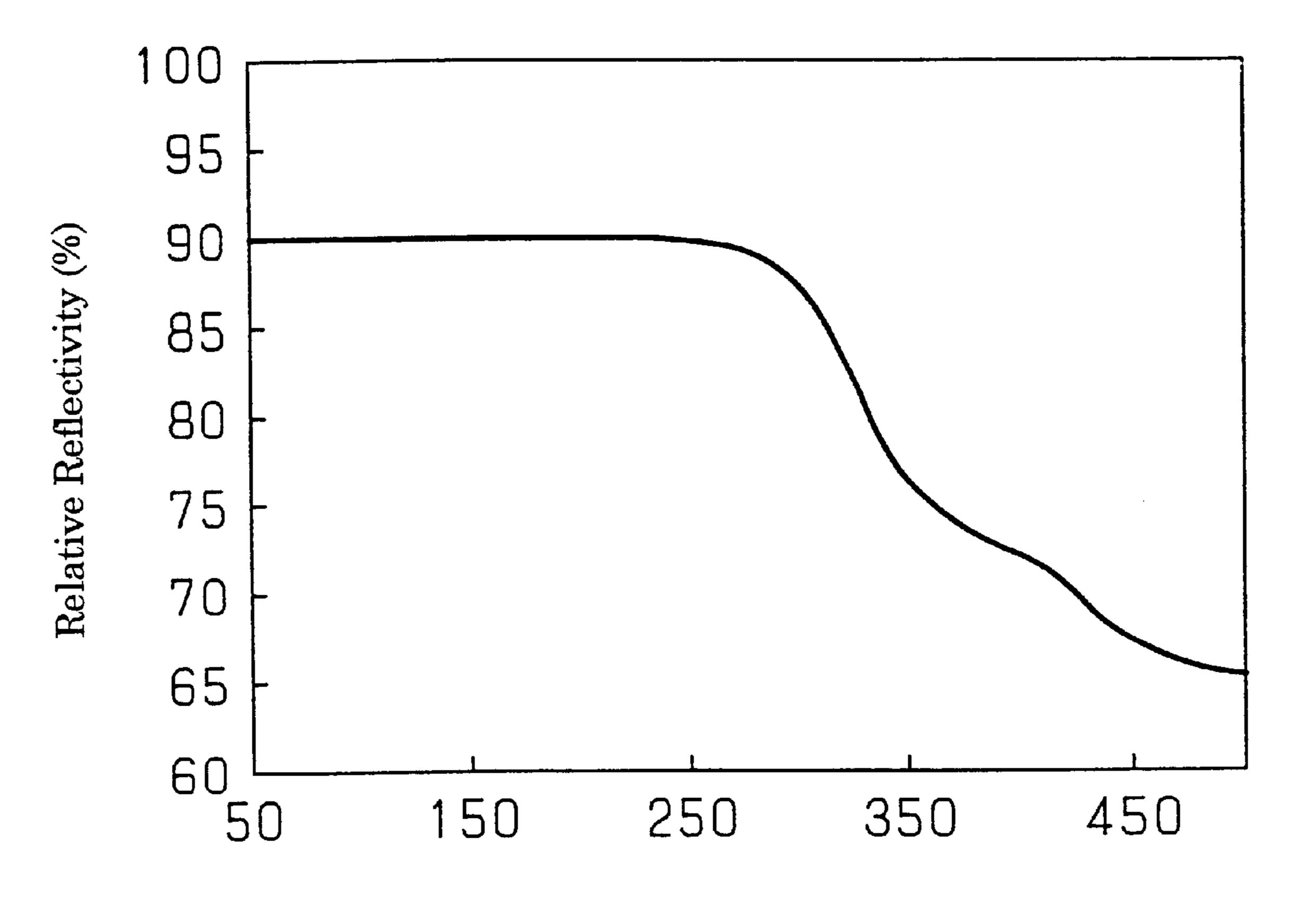
Aluminum Film Thickness (nm)
