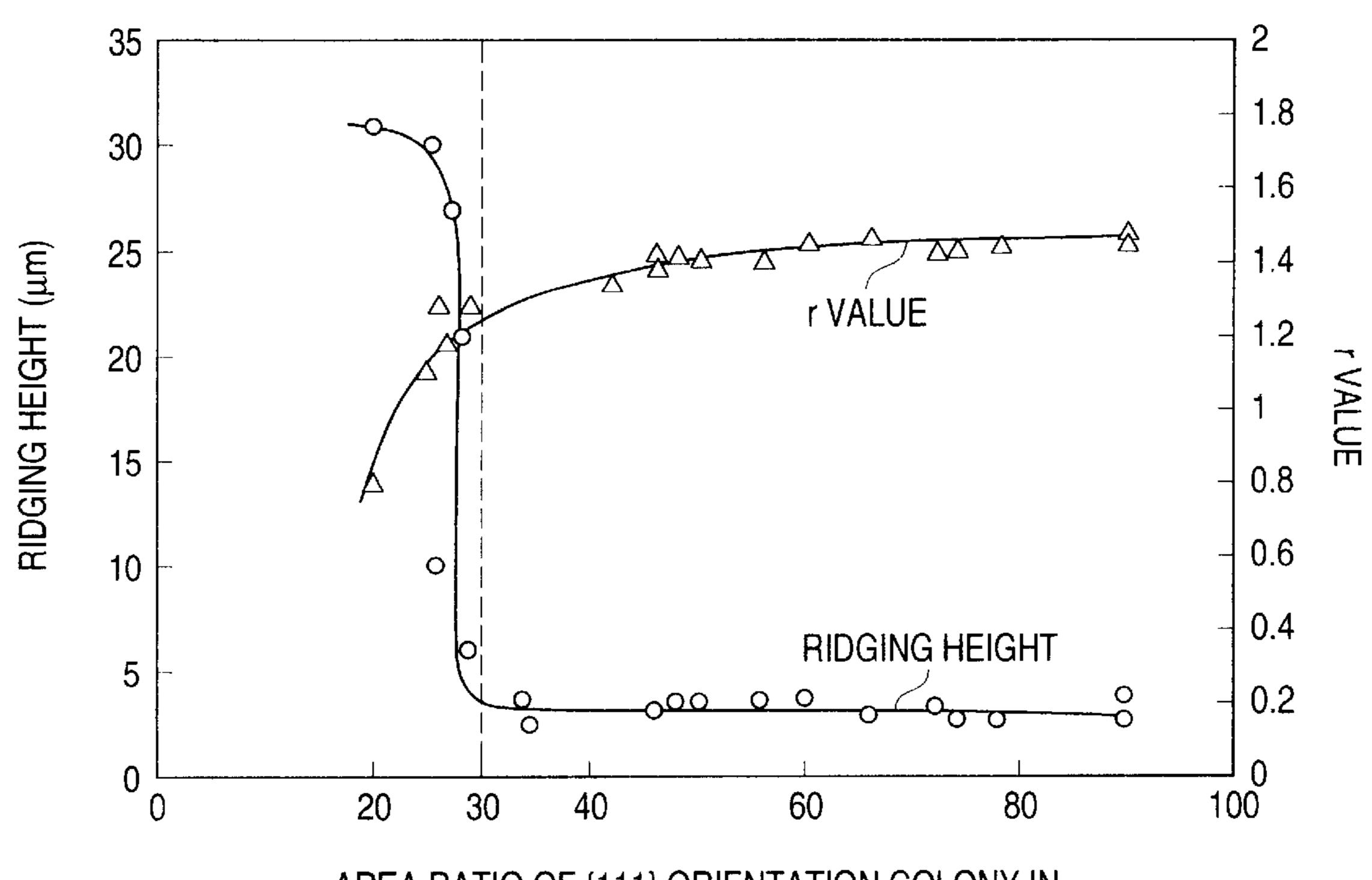
AREA RATIO OF {111} ORIENTATION COLONY IN 1/8 - 3/8 AND 5/8 - 7/8 REGION OF PLATE THICKNESS (%)
