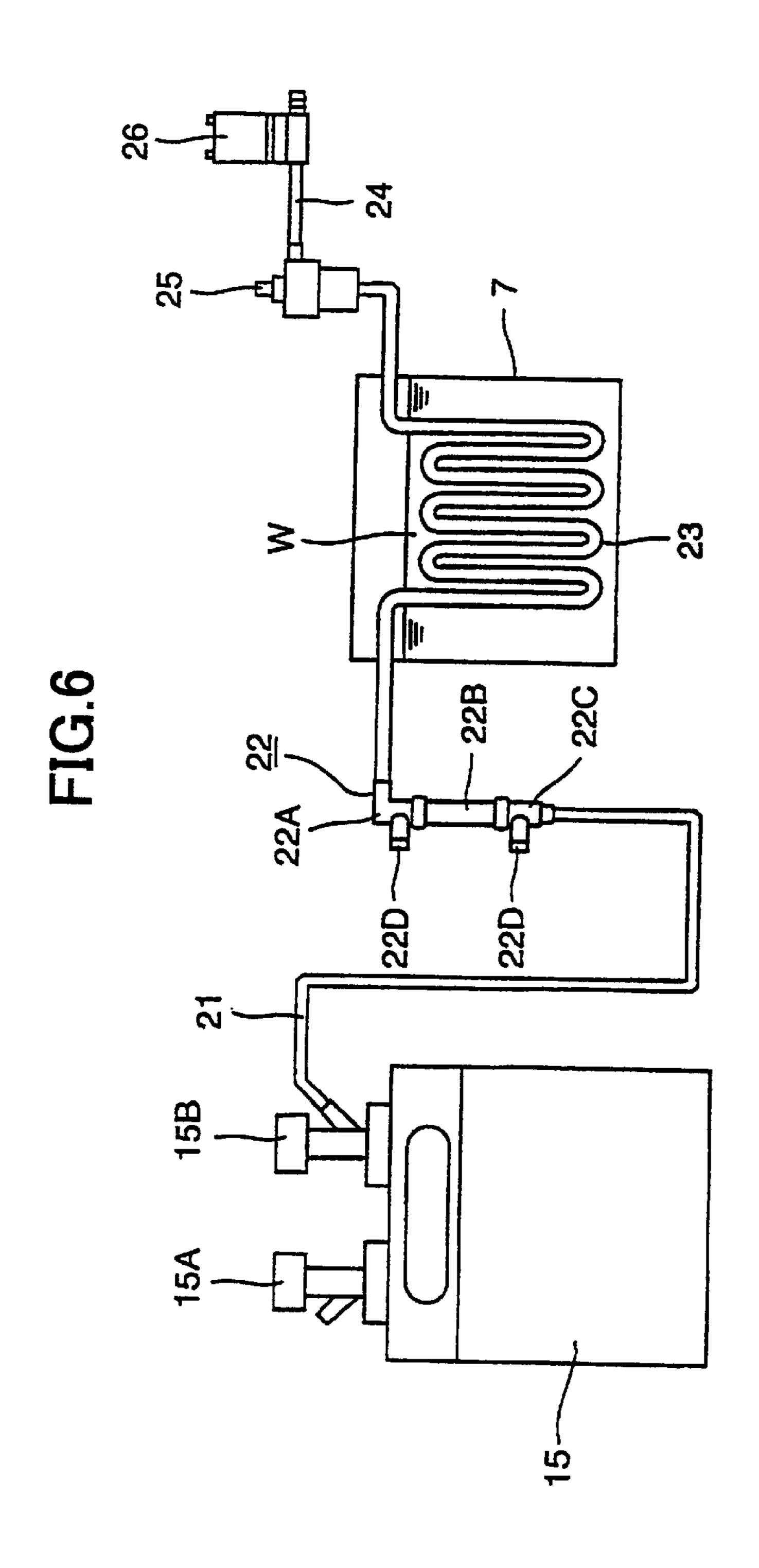
Cooling water vessel22CPipe connecting portionSyrup tank22DElectrode supporting portionGas Introduction portion23Cooling coilSyrup sending portion24PipePipe25Flow rate regulatorSold-out case26Electromagnetic valvePipe connecting portionWCooling waterMain body
