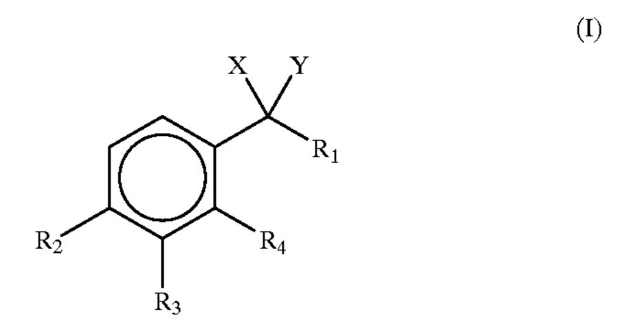
where X and Y independently of one another represent methoxy, ethoxy, propoxy, or butoxy groups, R<sub>1</sub> is a methyl, ethyl or propyl group, R<sub>2</sub> is hydrogen or an isopropyl, tert. butyl or methoxy group, R<sub>3</sub> is hydrogen or a methoxy group, and R<sub>4</sub> is hydrogen or a methyl group, and wherein at least one of R<sub>2</sub>, R<sub>3</sub> and R<sub>4</sub> is other than hydrogen.
