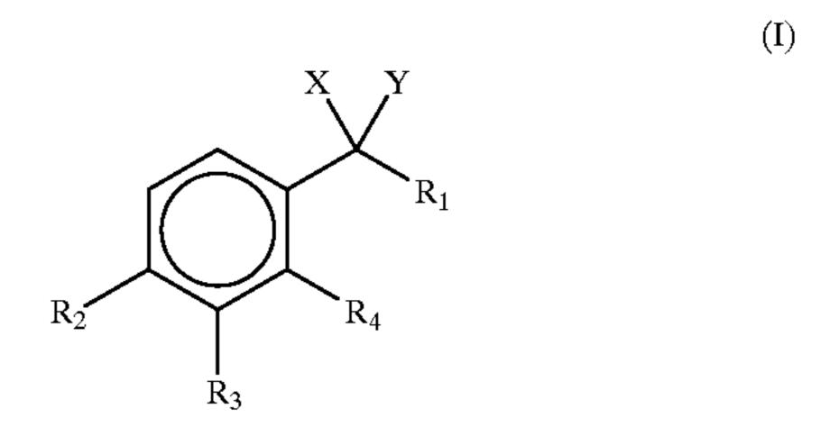
where X and Y independently of one another represent propoxy, or butoxy groups,  $R_1$  is a methyl, ethyl or propyl group,  $R_2$  is hydrogen or a methyl, ethyl, isopropyl, tert.butyl or methoxy group,  $R_3$  is hydrogen or a methoxy group, and  $R_4$  is hydrogen or a methyl group.
