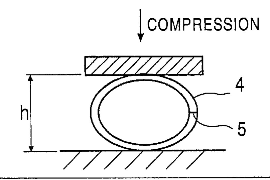
H: HEIGHT WHEN CRACKING OCCURS IN SEAM WELDED PORTION
