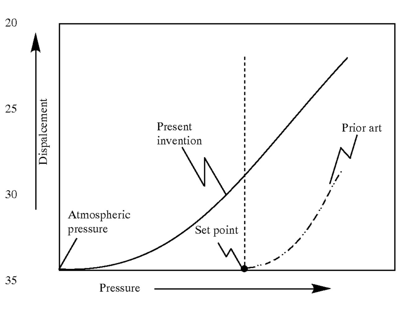
It is thus an object of the present invention to provide a tire gauge apparatus which relies on pressure equilibration rather than on a mechanical spring to produce a tire pressure reading.
