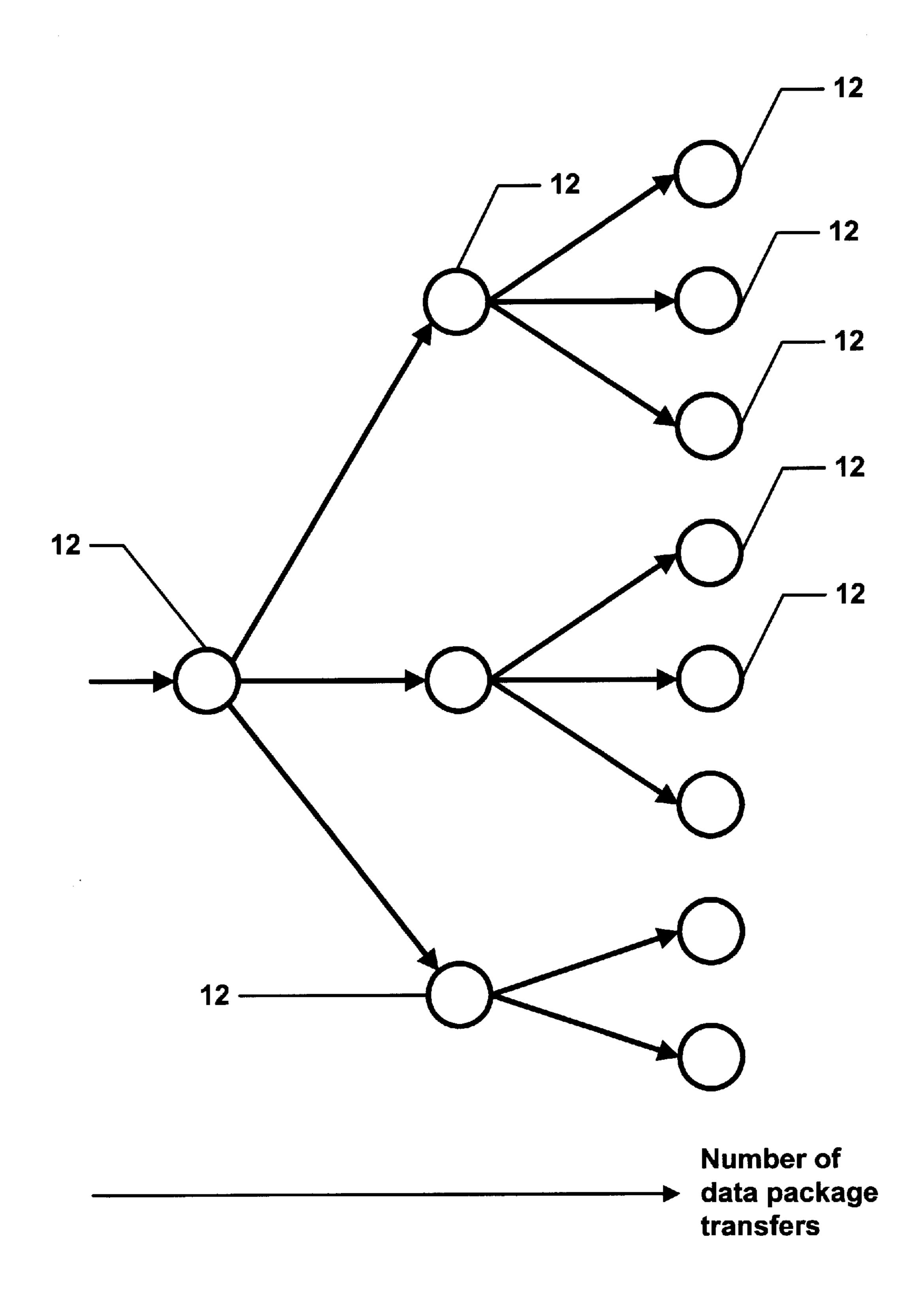
FIGURE 3: Tree-shaped data-flow (optimal)
