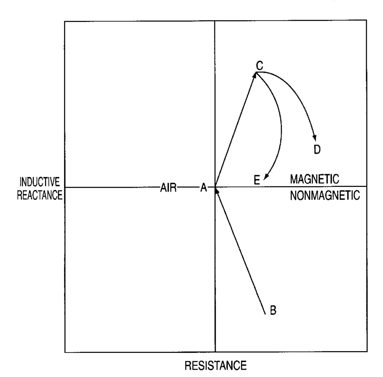
LIFT-OFF LOCUS FOR NON-MAGNETIC MATERIAL PERMEABILITY LOCUS FOR MAGNETIC MATERIAL CONDUCTIVITY LOCUS FOR MAGNETIC MATERIAL
