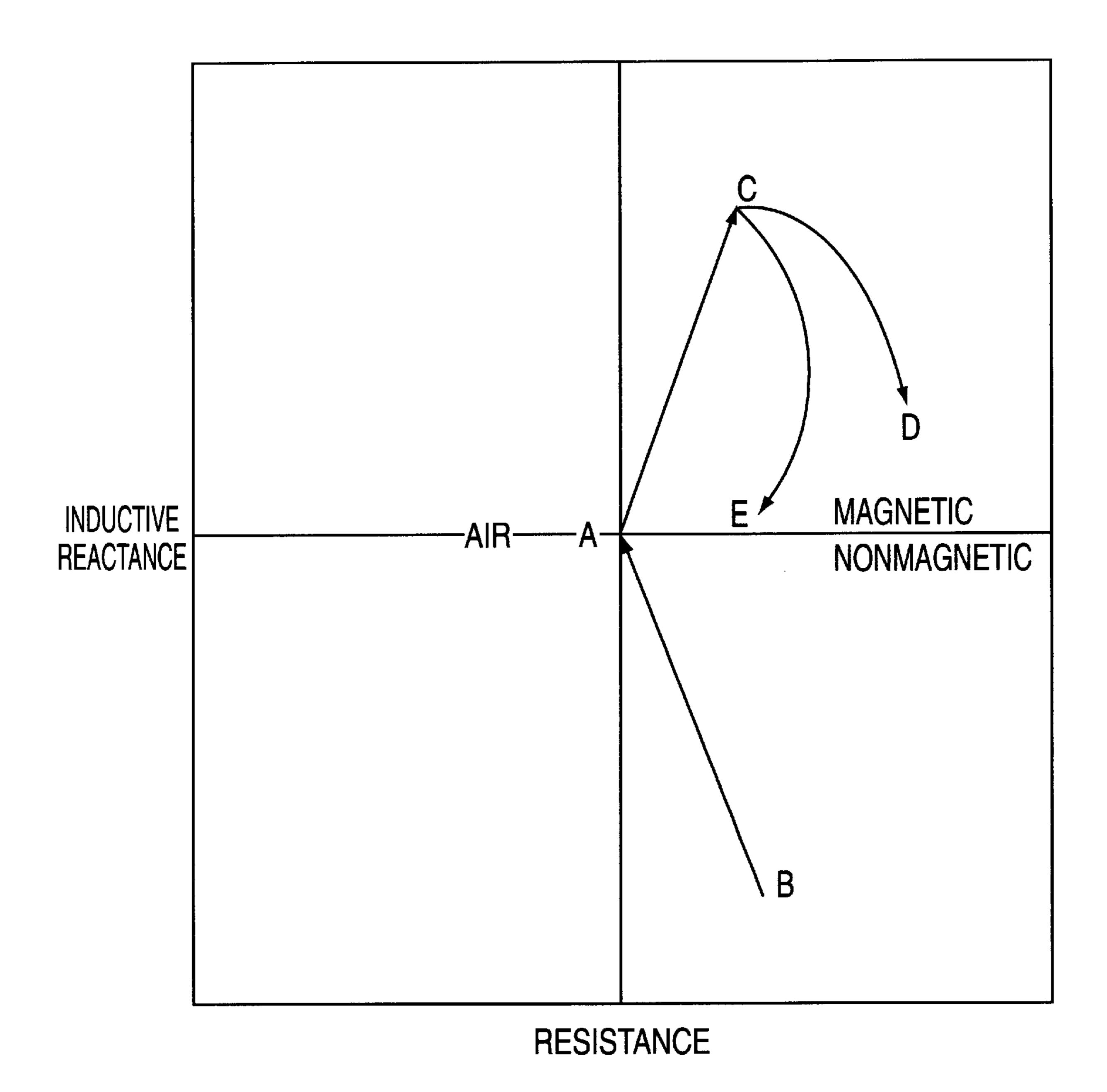
B-A LIFT-OFF LOCUS FOR NON-MAGNETIC MATERIAL
