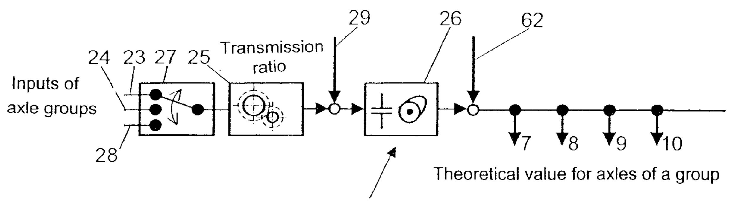
Dynamic change from electronic curved disc profiles to the work synchronous engagement and disengagement of axle groups
