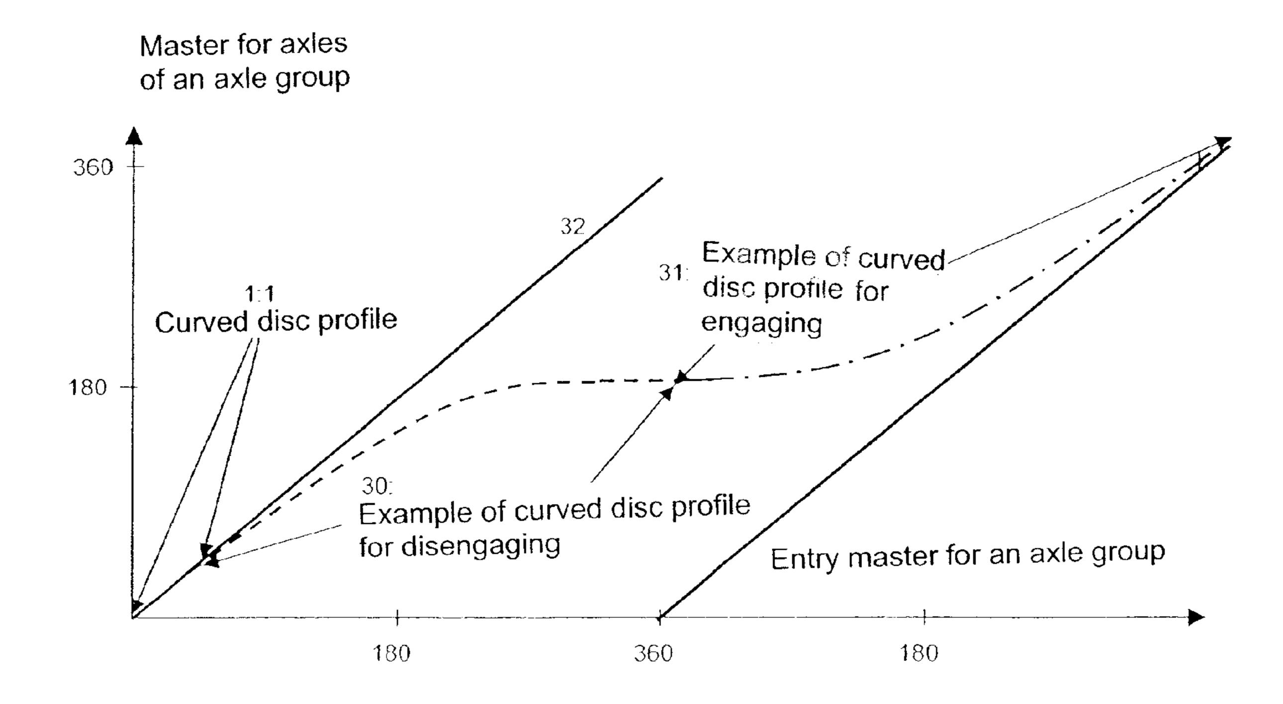
Fig. 3: Electronically simulated curved disc profile for continuous use (1:1) and an example of two curves for stroke synchronous engaging and disengaging of a servo axle group
