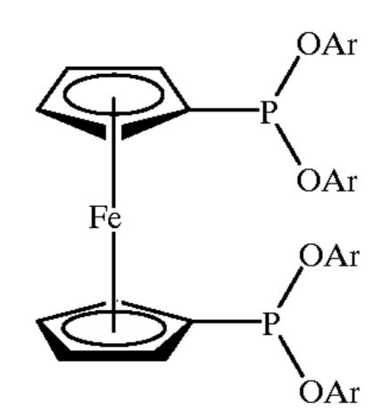
wherein the Ar groups are either the same or different unbridged organic aromatic groups such as substituted or unsubstituted phenyl, substituted or unsubstituted naphthyl, mixtures thereof or the like are disclosed. The ligands in combination with a Group VIII metal or Group VIII metal compound are particularly useful in a hydroformylation process for reacting an ethylenically unsaturated compound to produce linear alkenals at high selectivity.
