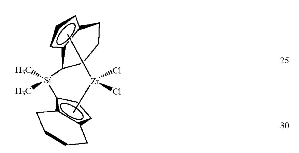
dimethylsilylbis(2-methyl- 1-indenyl)zirconium dichloride;
