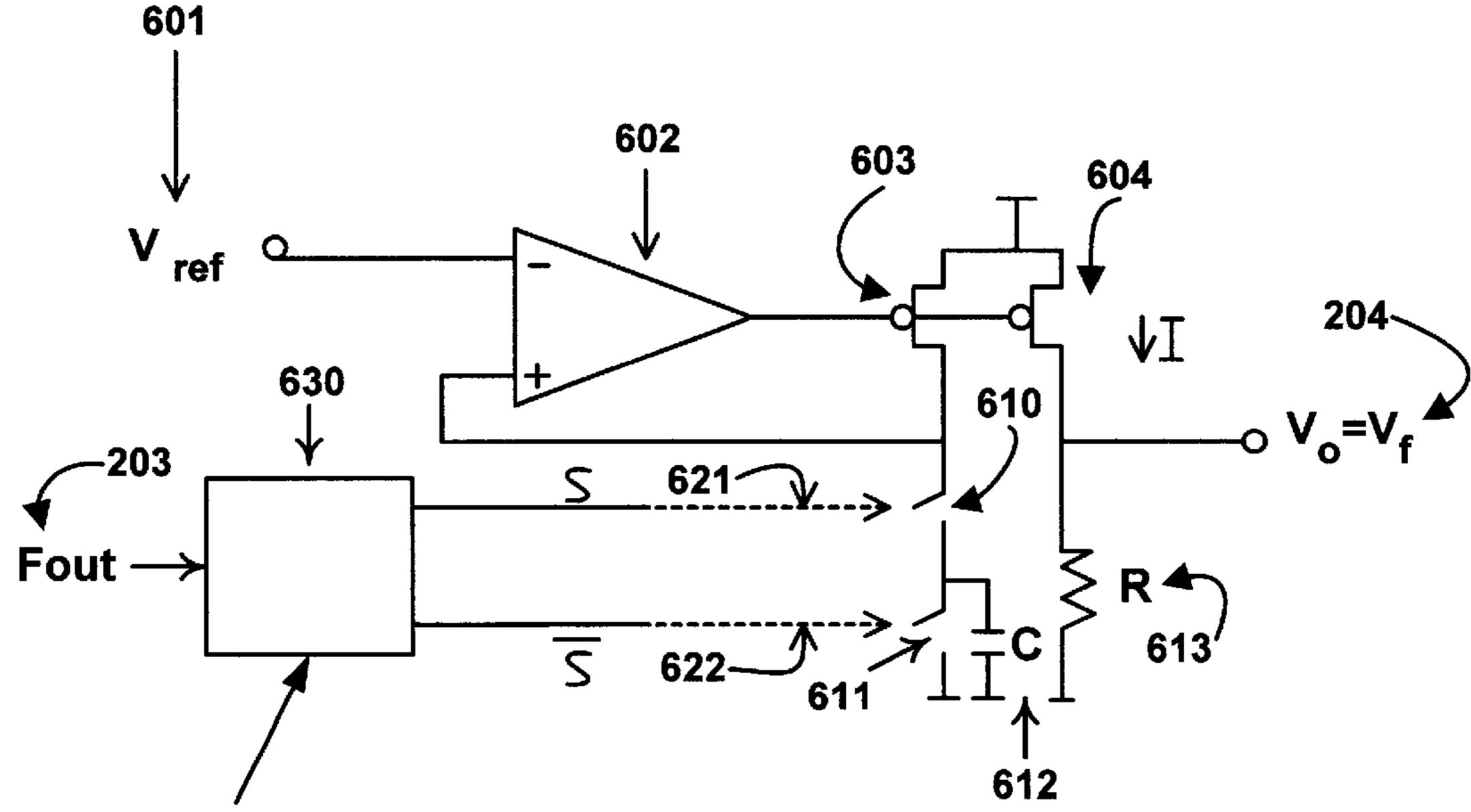
Logic for rapidly opening and closing switches 610 and 611 in response to the frequency of Fout
