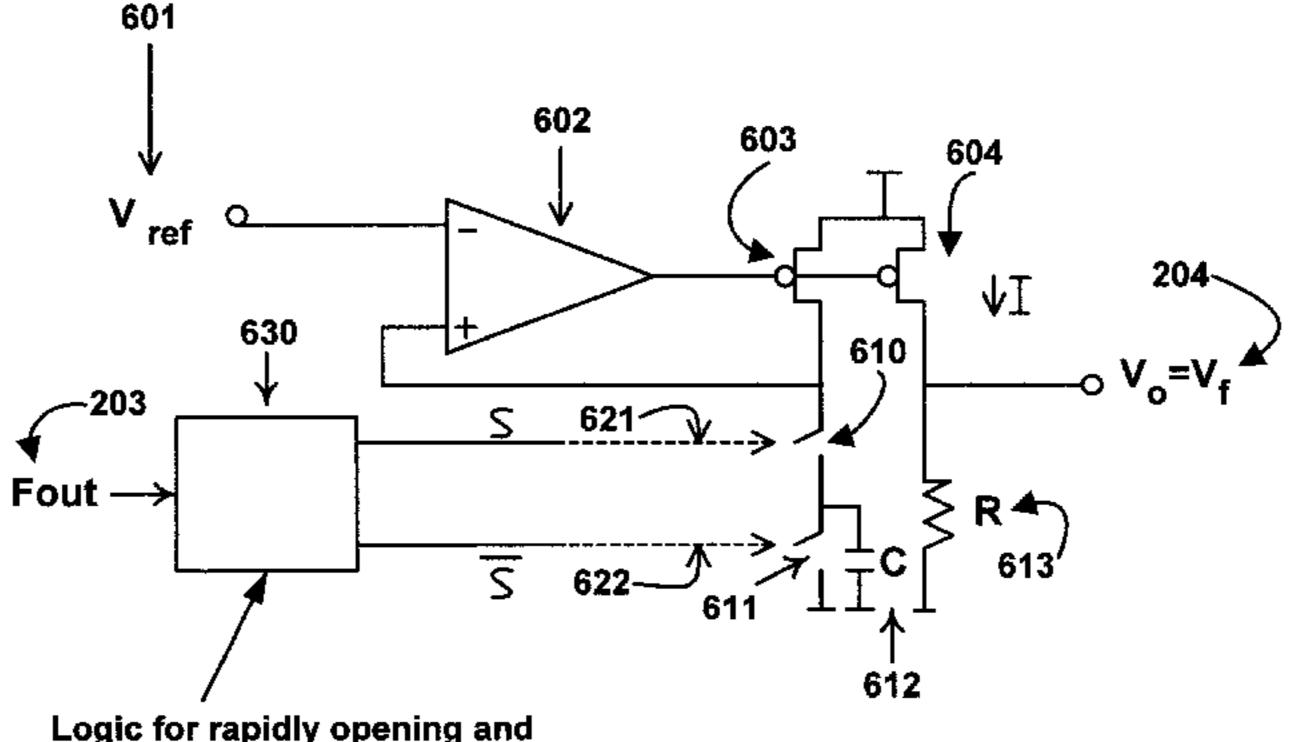
Logic for rapidly opening and closing switches 610 and 611 in response to the frequency of Fout
