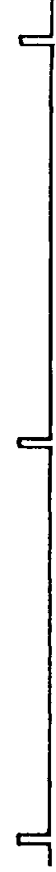
OUTPUT OF TIMING SIGNAL FORMING CIRCUIT
