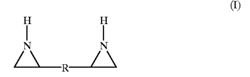
where R is any linking polymer of any length. For example, R may be 3–50 carbon atoms in length, or may include branched carbon chains or other functional groups.
