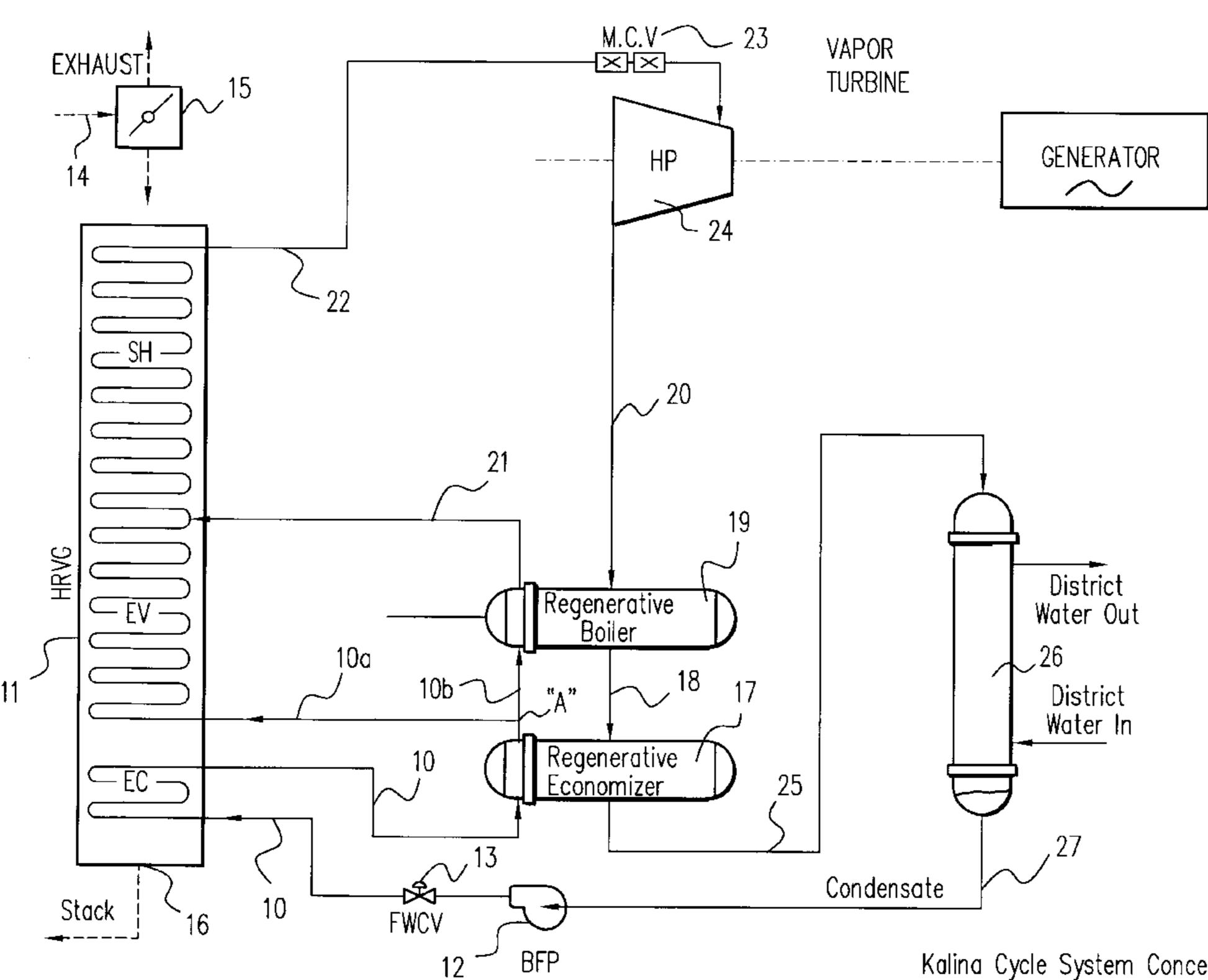
Kalina Cycle System Conceptual Diagram For CC Power Plants With District Heating
