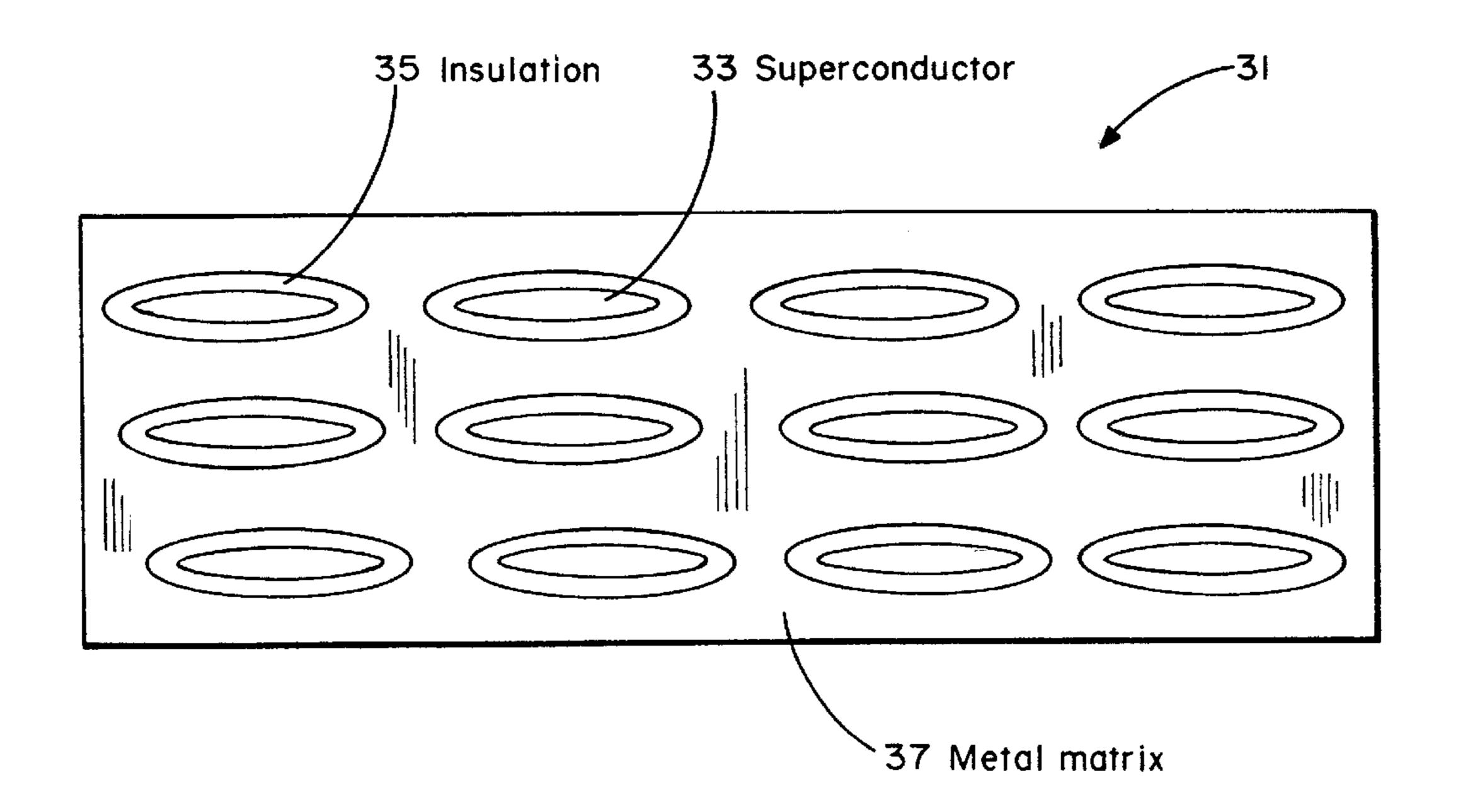
Low AC loss superconductor by decoupled filaments using sol-gel insulation.
