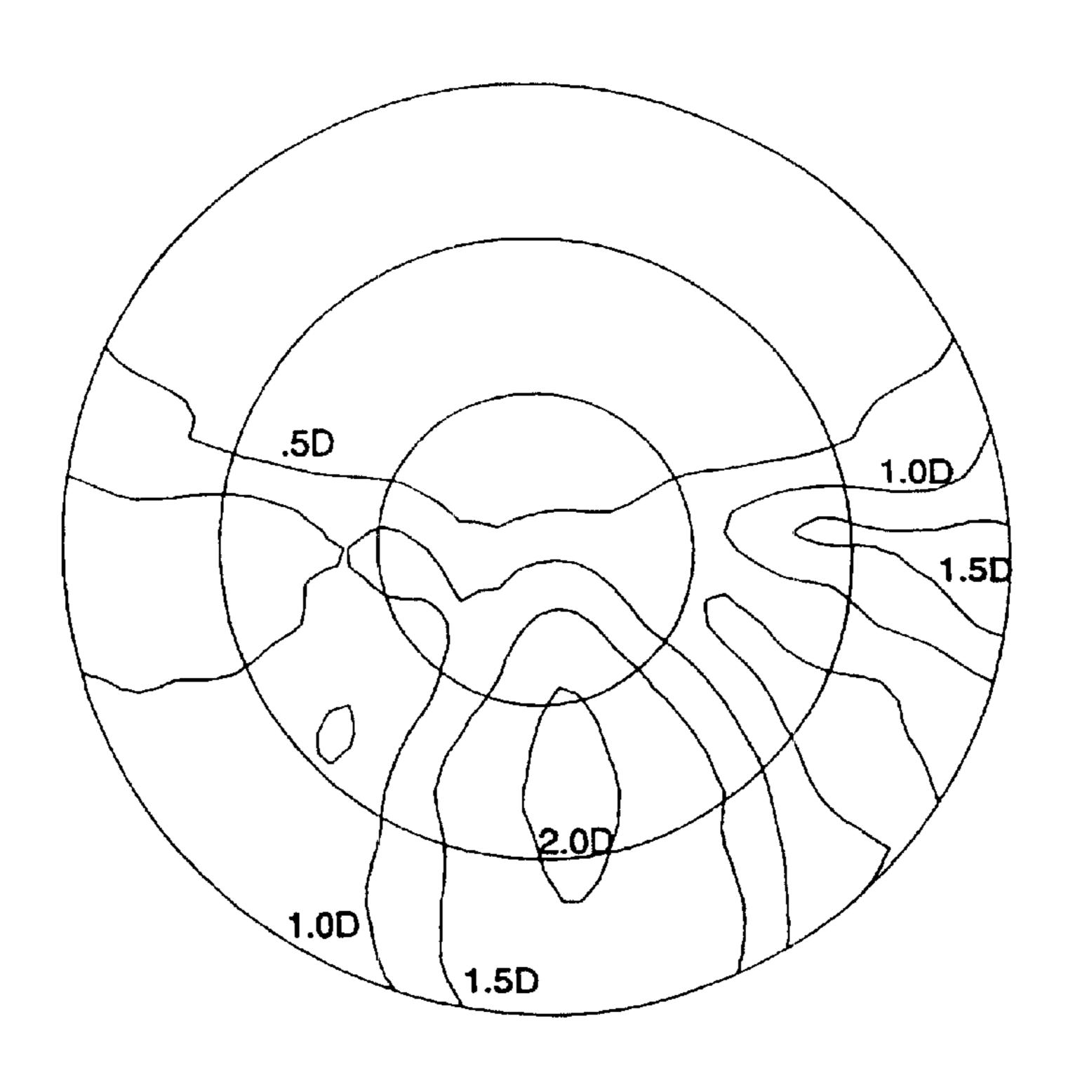
The present invention relates to a progressive ophthalmic lens and in particular to a progressive ophthalmic lens designed to reduce the rate of juvenile myopia progression, and to a process for producing such lenses.
