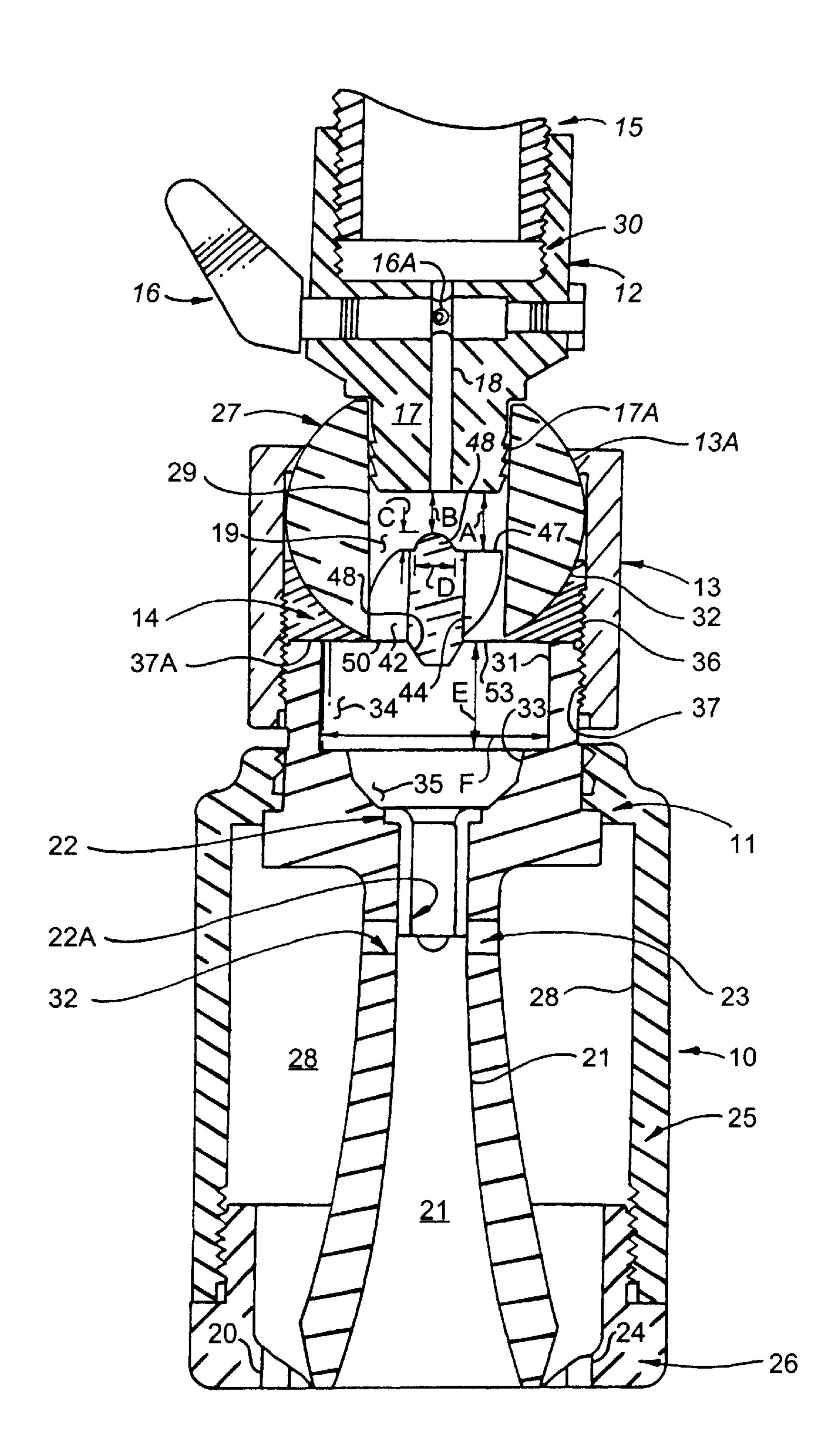
More particularly, the invention pertains to a water conserving shower head which operates quietly, produces a 5 relatively full pattern of water droplets, and in use consumes a minimal amount of water.
