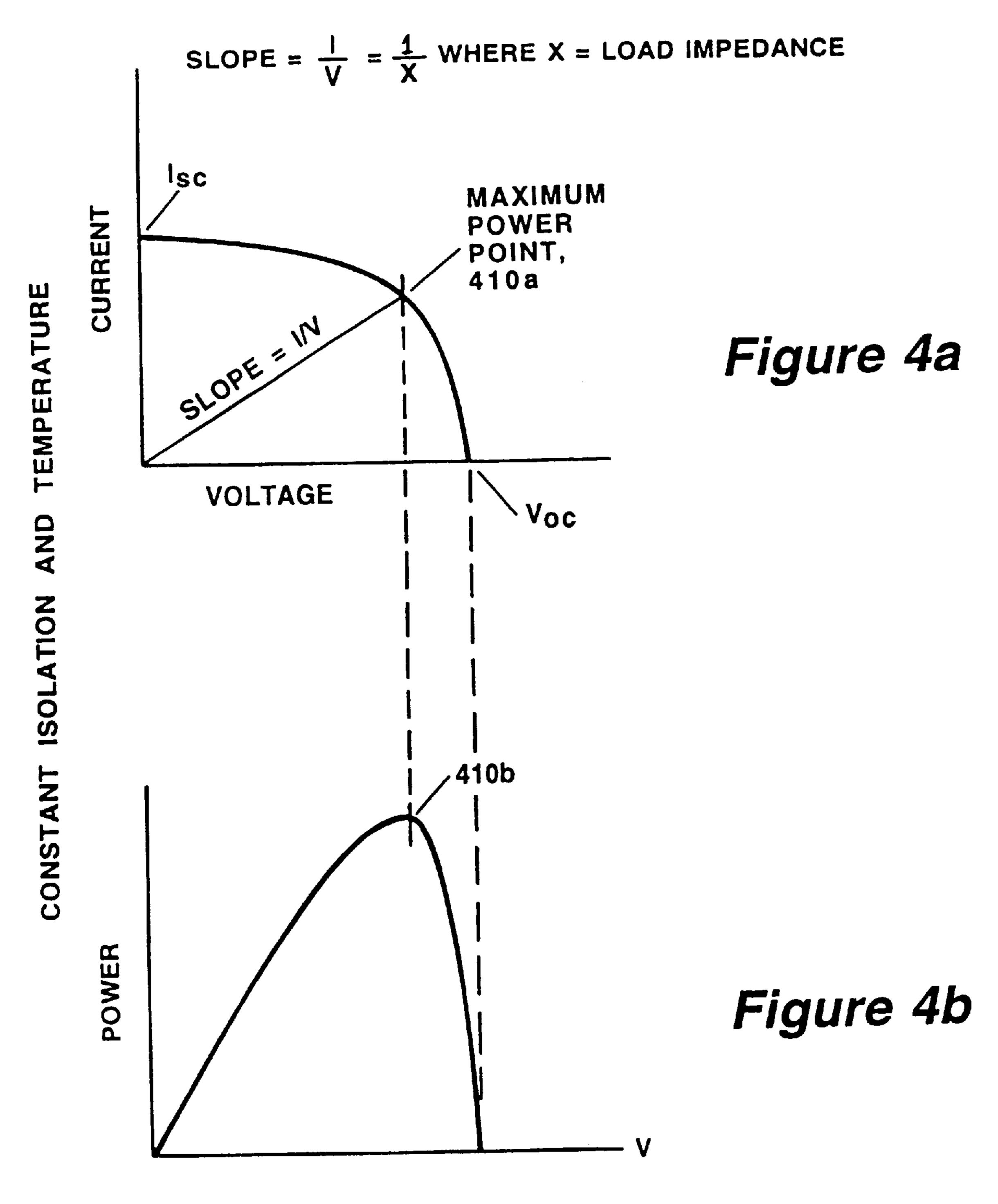
Isc = ARRAY SHORT CIRCUIT CURRENT Voc = ARRAY OPEN CIRCUIT VOLTAGE
