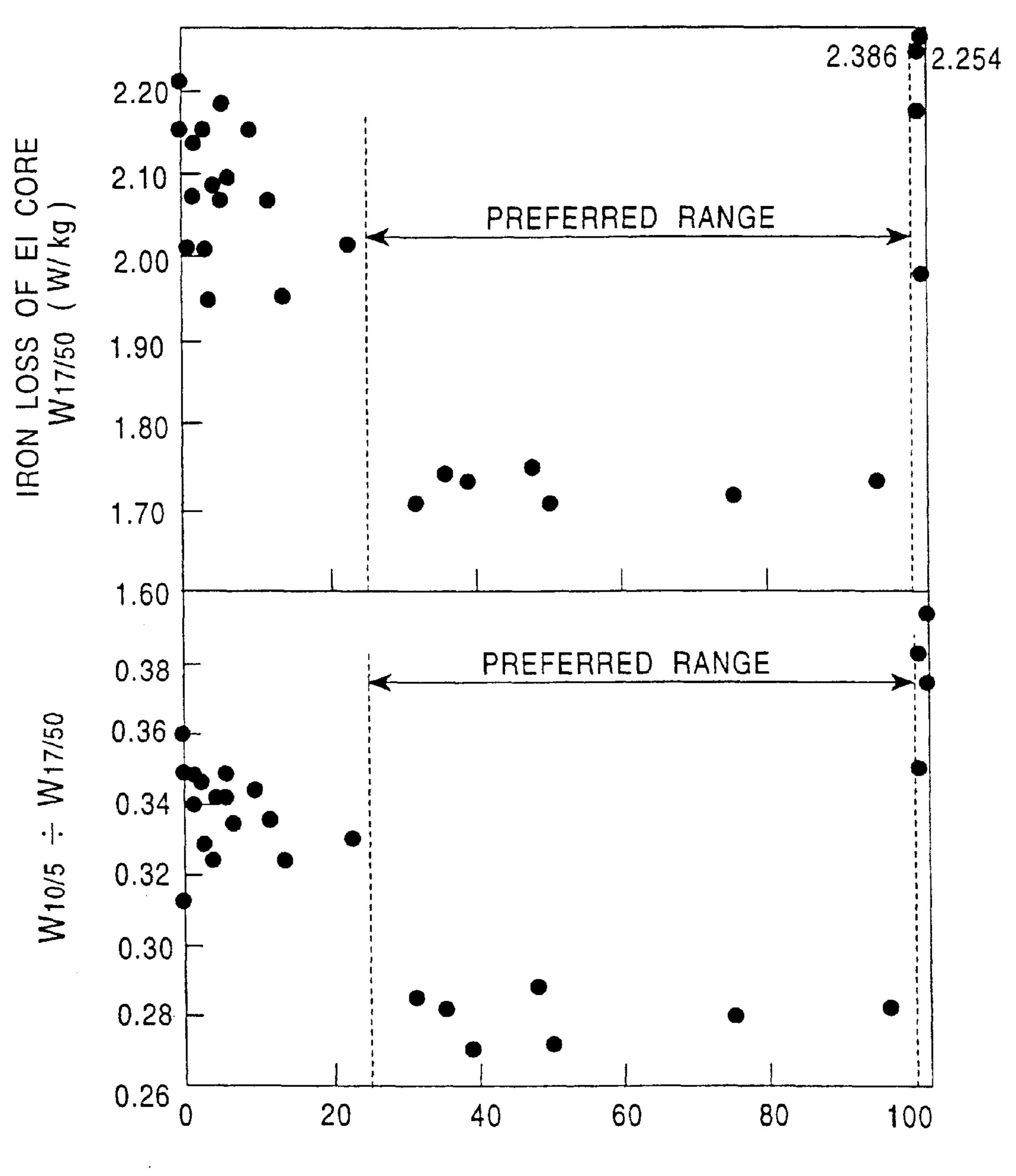
PROPORTION IN NUMBER OF CRYSTAL GRAIN OF BELOW 1 mm IN GRAIN DIAMETER (%)
