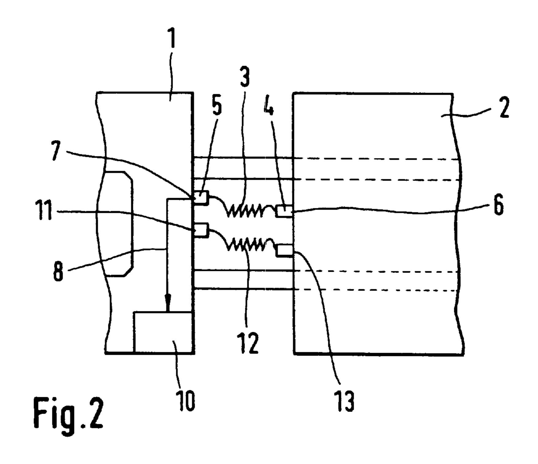
DEVICE FOR DETECTING THE MEASURED QUANTITIES OF A DRIVE VEHICLE AND/ OR THE MEASURED QUANTITIES OF A TRAILER OR SEMITRAILER MECHANICALLY LINKED TO A DRIVE VEHICLE, IN PARTICULAR A TRAILER OR SEMITRAILER
