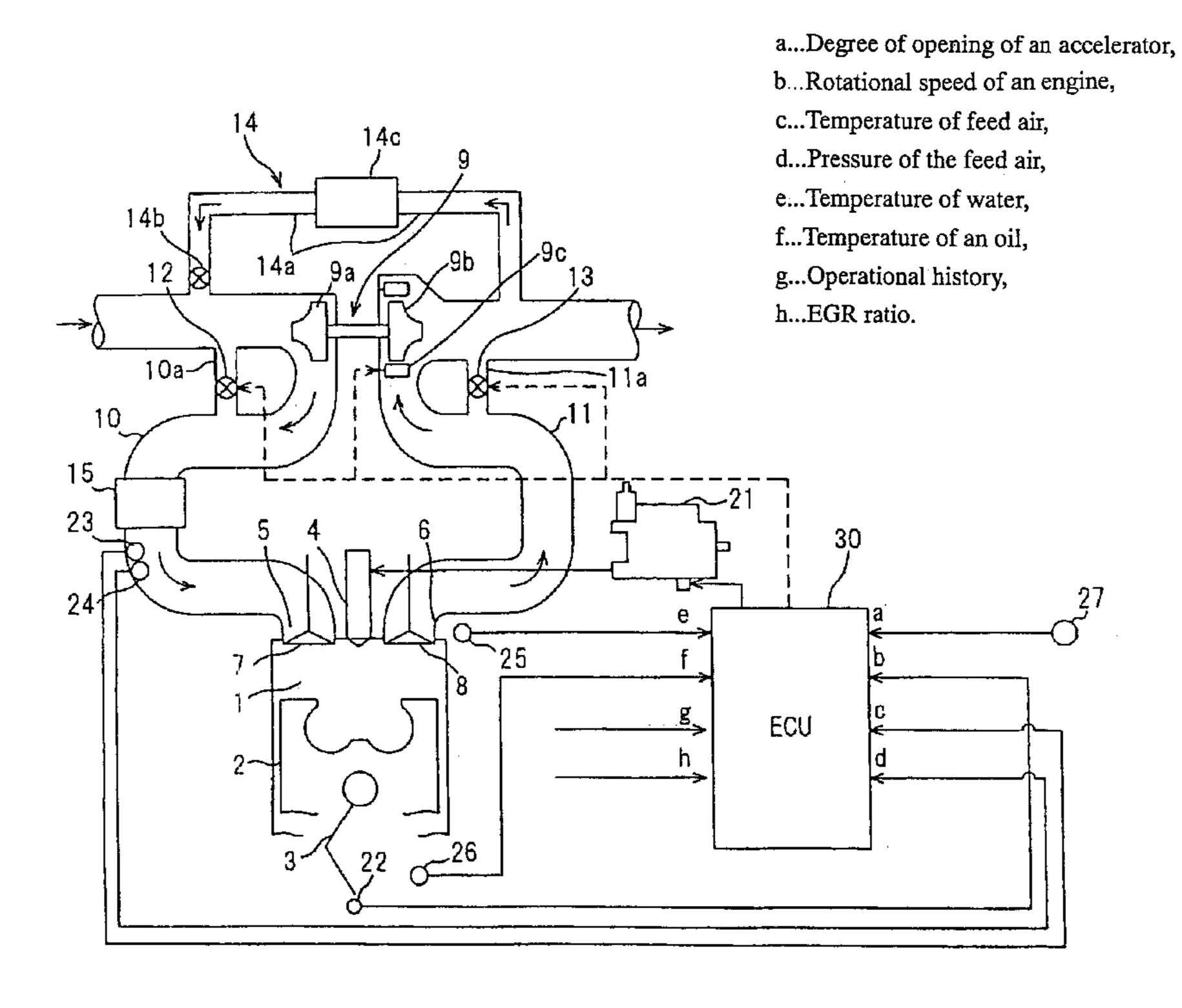
accelerator, b...Rotational speed of an engine, a...Degree of opening of an c...Temperature of feed air, d...Pressure of the feed air, e...Temperature of water, f...Temperature of an oil, g...Operational history, h...EGR ratio. D0∫ 25 ഹ -
