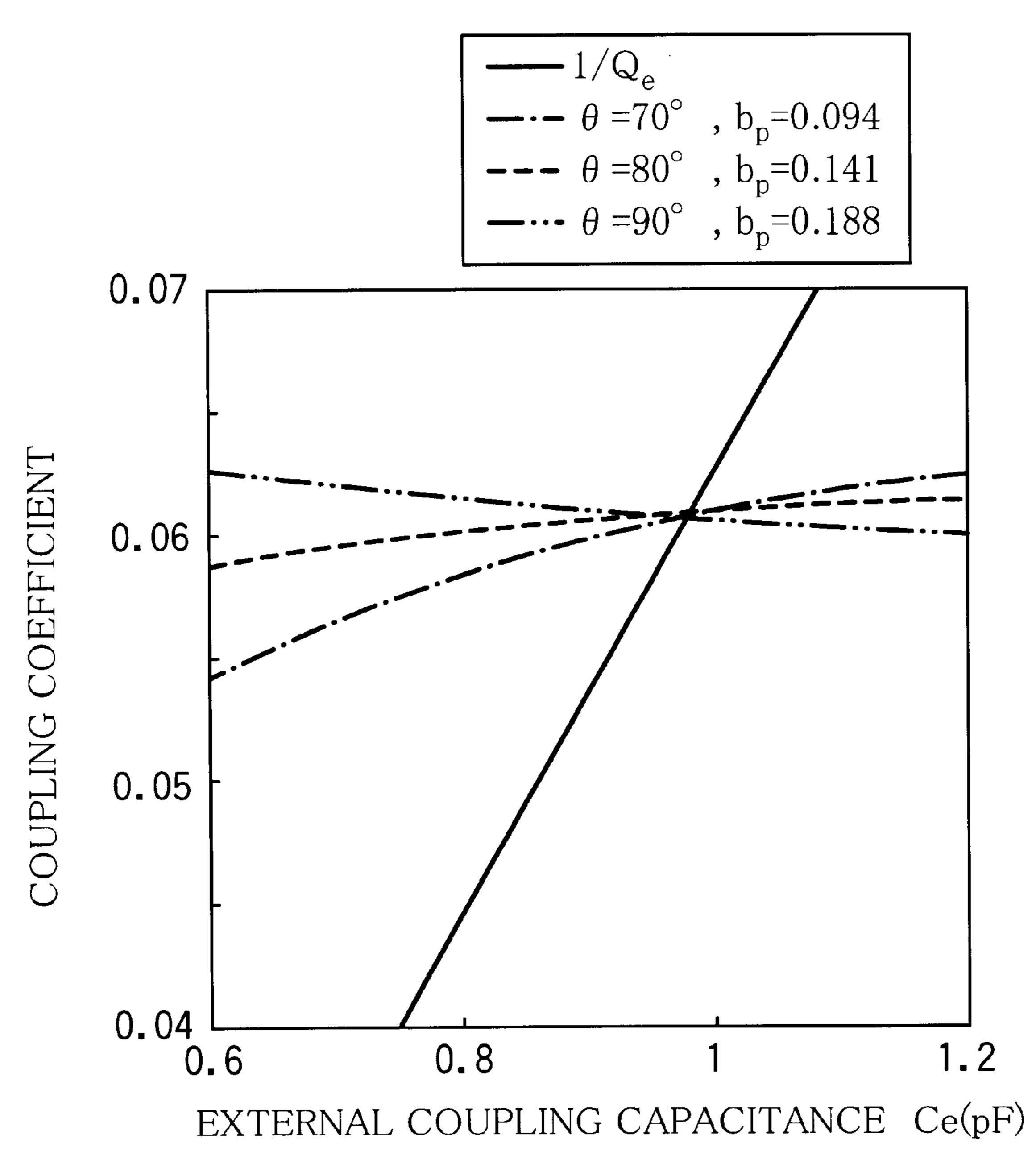
(f=2.08GHz,y<sub>a</sub>=0.028336 S) Q<sub>e</sub>:External Quality Factor
