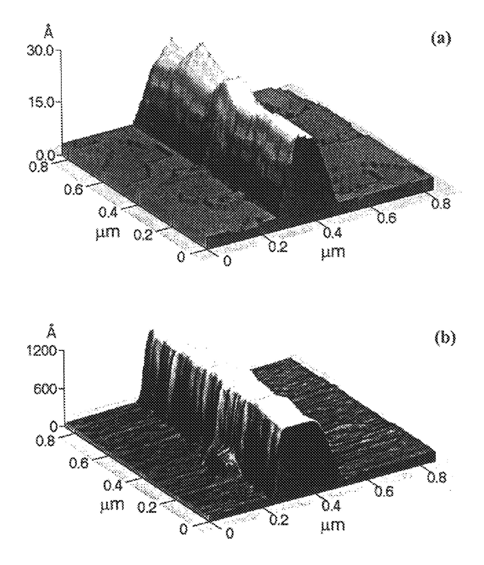
Figure 7. Close up AFM profiles of (a) oxide line on (110) silicon and (b) same line after anisotropic wet chemical etching in TMAH.
