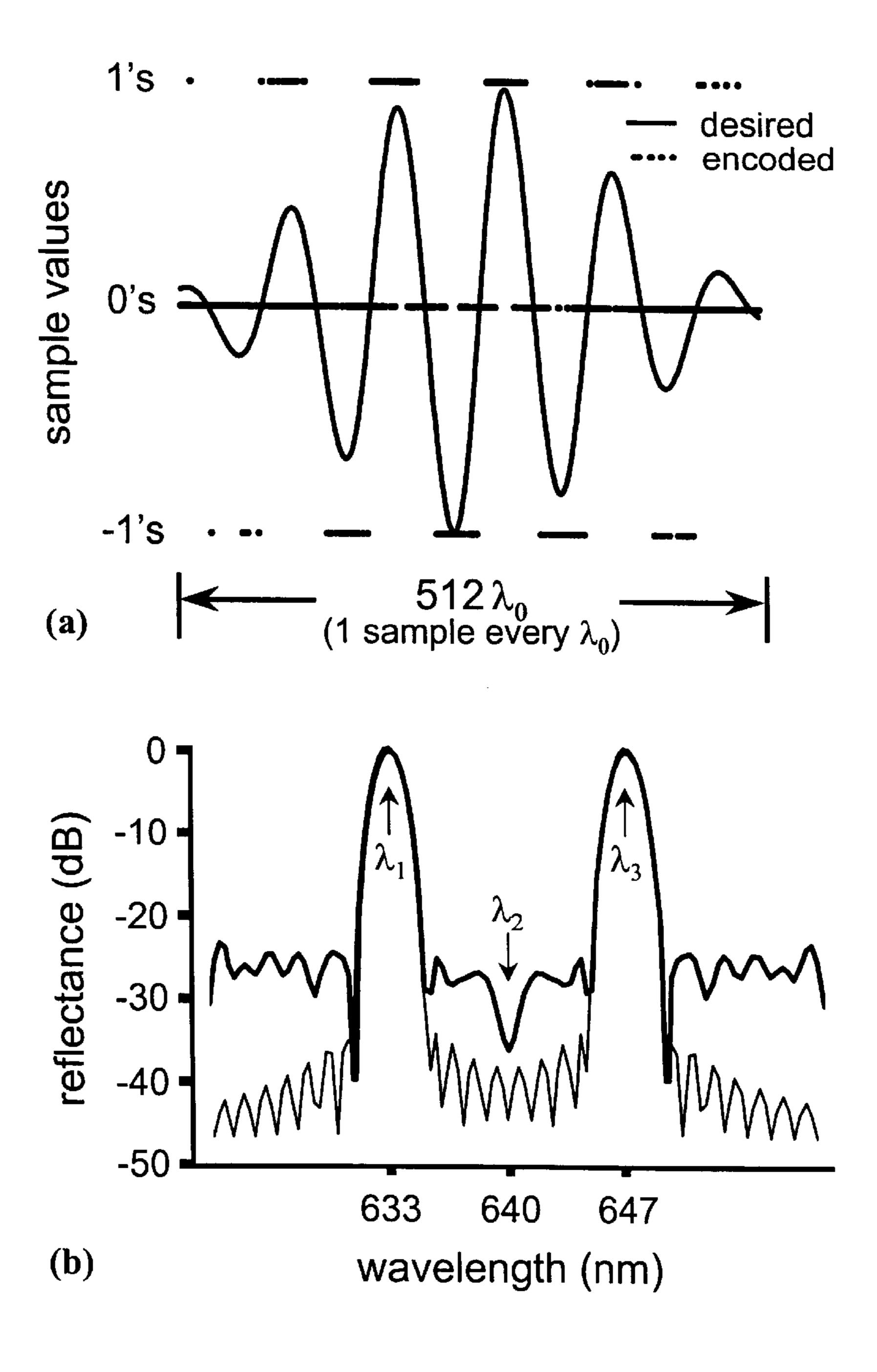
Figure 2. Pseudorandom encoding of dual passband filter. (a) Desired real-valued reflectances and the desired function encoded with the three available values -1, 0 and 1. (b) The reflectance power spectra derived from the Fourier transforms of the temporal functions in (a). The thin line is the spectrum for the desired function and the thick line is the spectrum for the encoded function.
