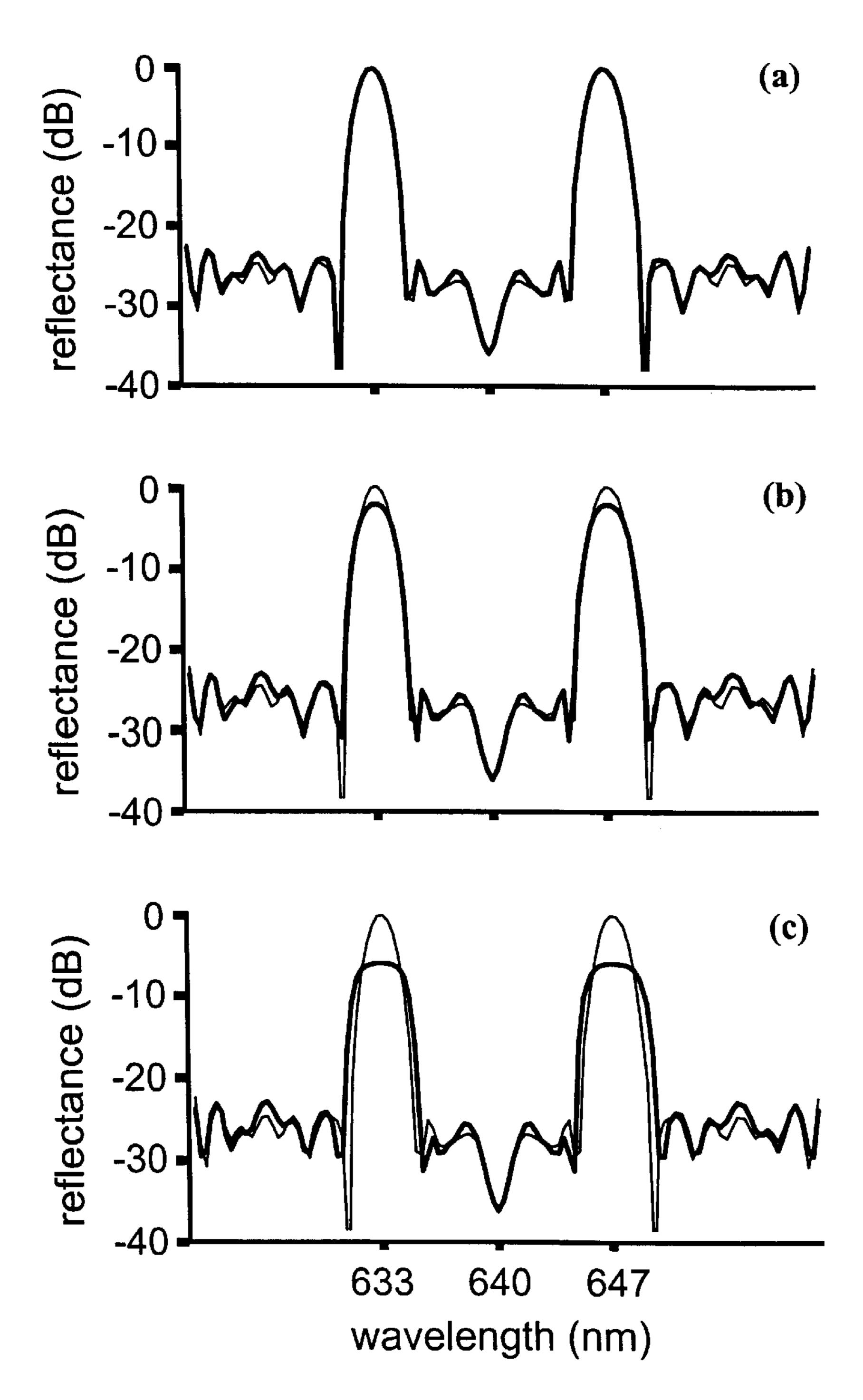
Figure 4. Reflectance spectra for the dual passband filter design. The DL analyses (thick lines) are shown for filter insertion loss (i.e. peak intensity reflectance at centerband) of (a) 0.068, (b) 0.532 and (c) 0.917. The spectrum for the dual passband design from Fig. 2 is also replotted (thin line) for comparison. The reflectance spectra are normalized so as to bring their sidelobe structure into correspondence with the design spectrum.
