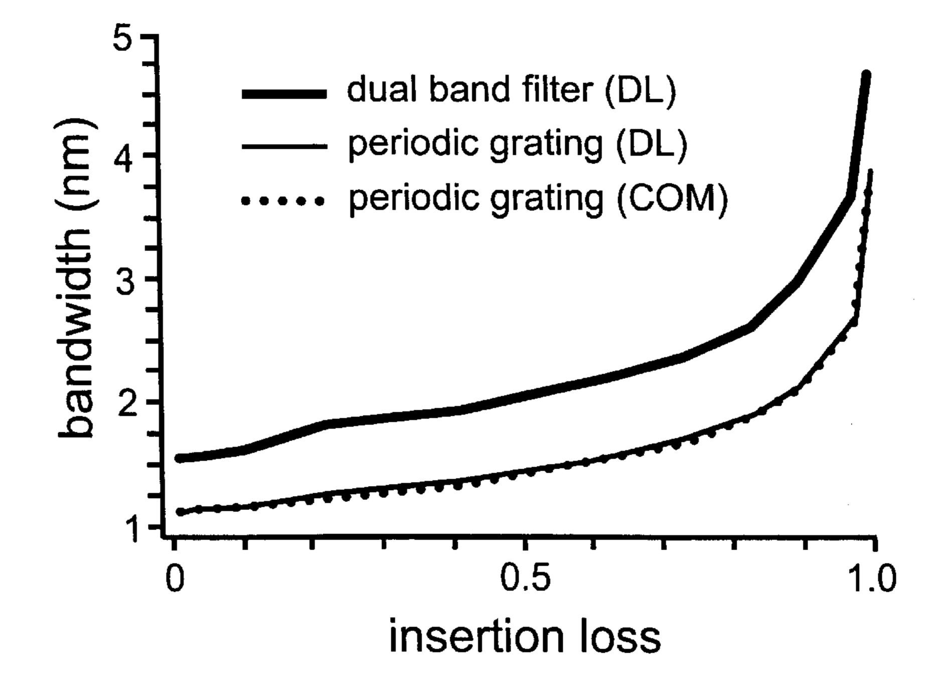
Figure 3. Bandwidth at -3 dB of peak intensity for a single passband (512 period) grating filter and the dual passband grating filter as a function of filter insertion loss. The correspondence between the COM (coupling of modes) and DL (discrete layer) analyses for the periodic structure indicates the validity of the DL analysis for the analysis of the non-periodic dual passband filter.
