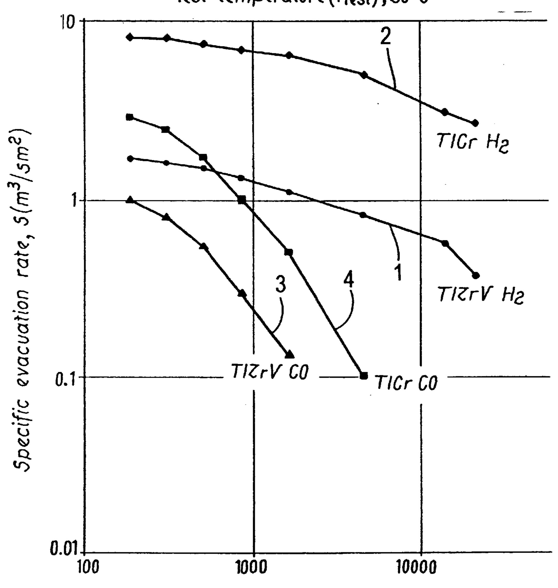
Quantity of absorbed gas, Q(Pa m³/m²)
