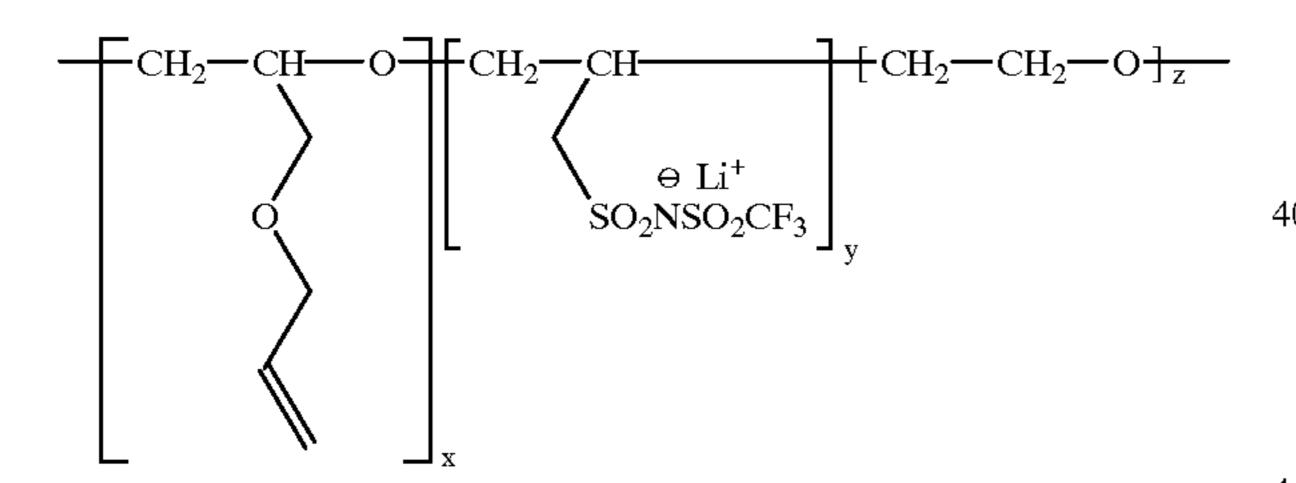
This polymer enables to prepare gelled polymer electrolytes with fixed anions, the polymer ensuring a double matrix functionality enabling to obtain the gel of polyelectrolytes. It may be crosslinked during the process of preparing an electrochemical system containing same.
