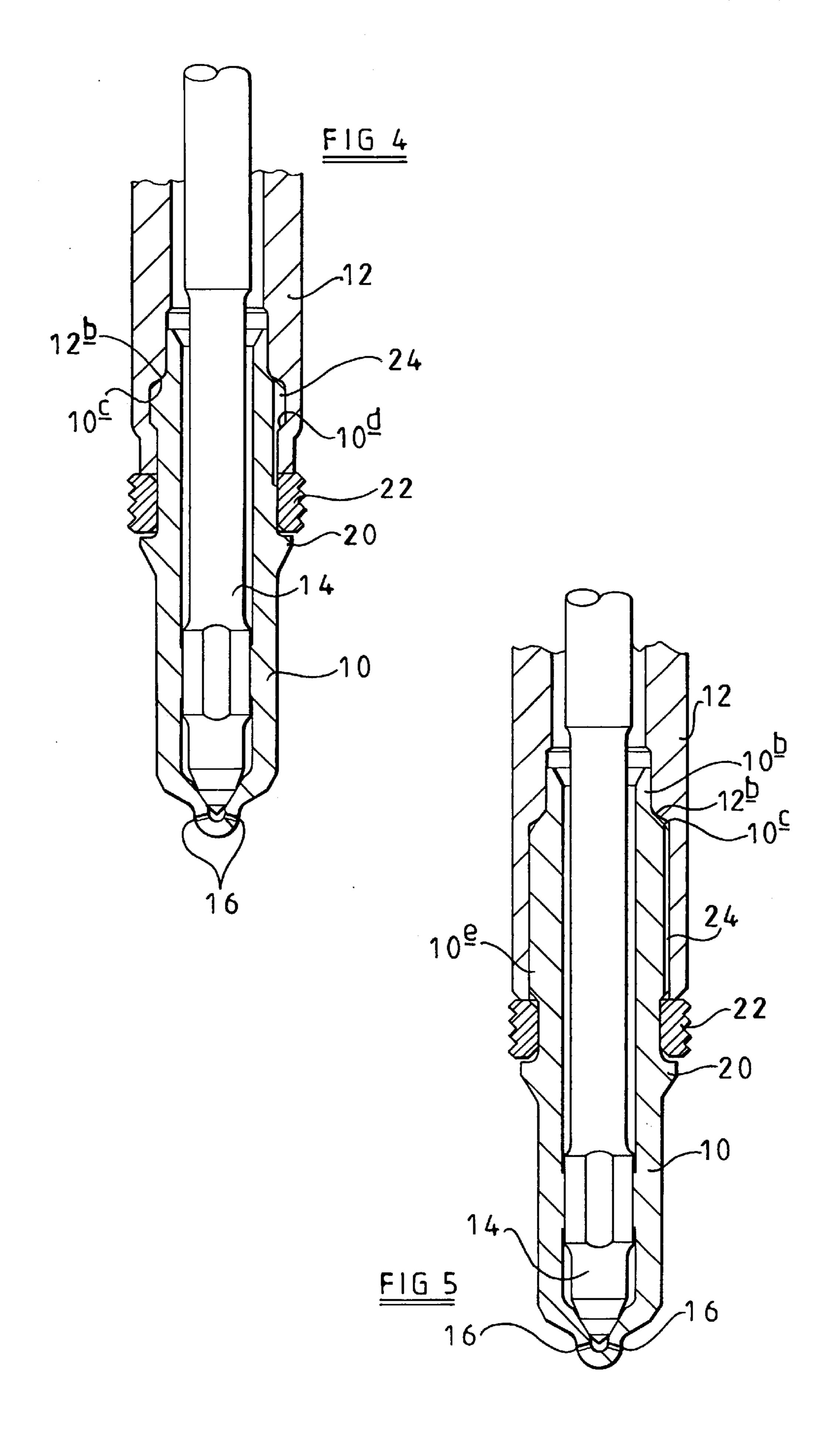
This invention relates to a nozzle for a fuel injector intended for use in delivering fuel, under pressure, to a cylinder of a compression ignition engine.
