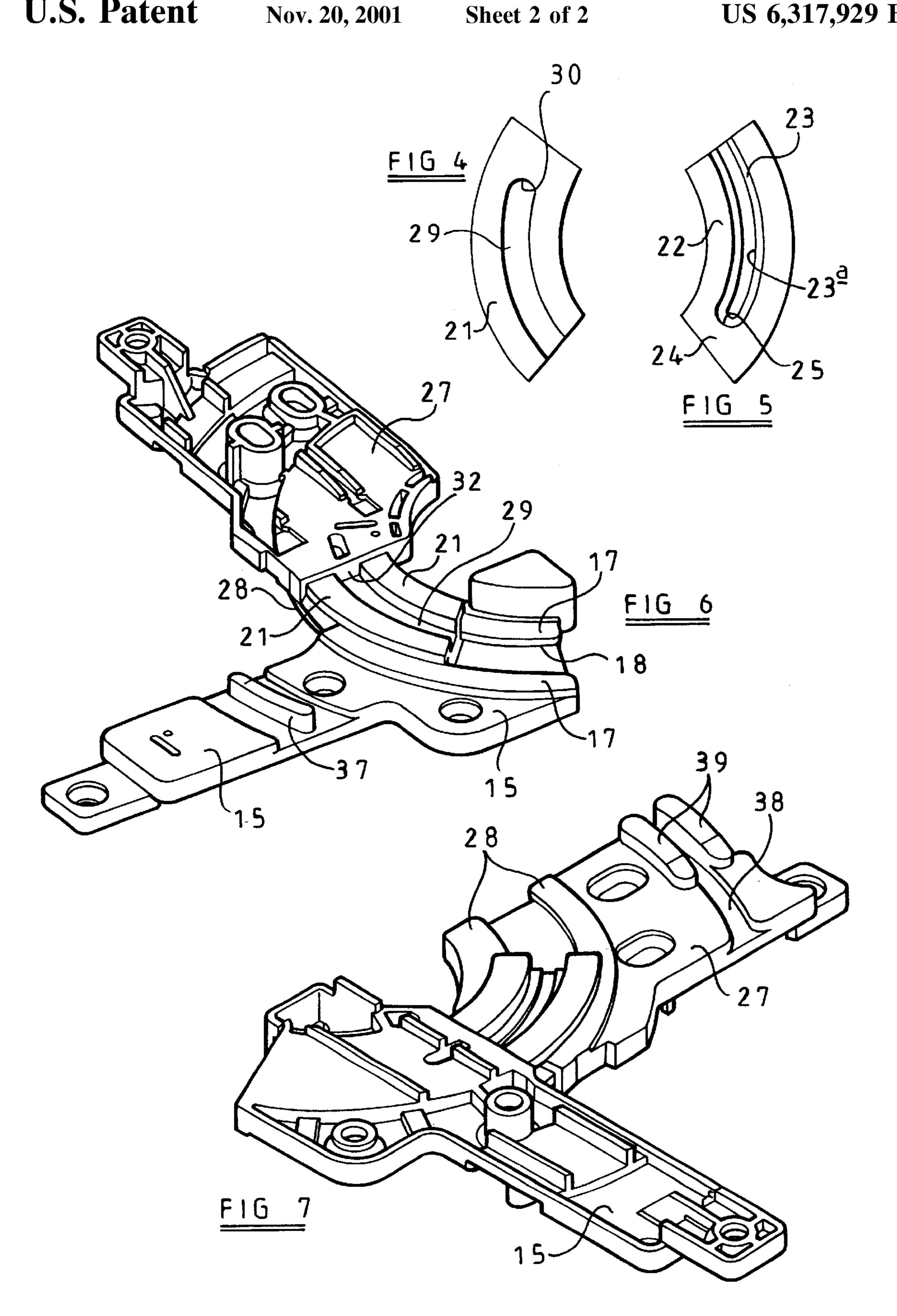
The invention relates to hinges and in particular to friction hinges for windows,
