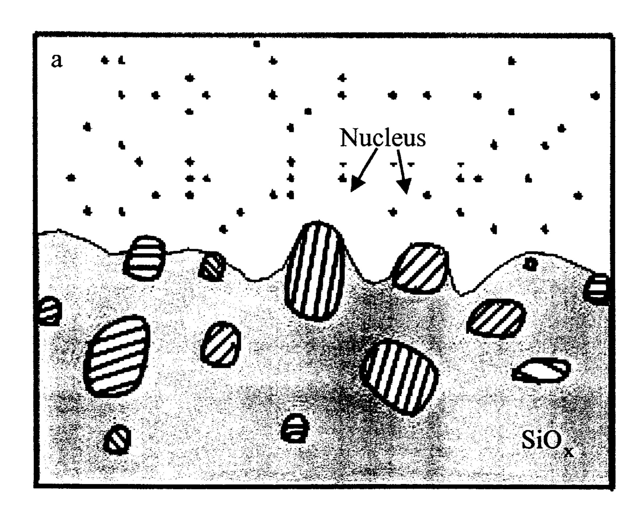
Nucleation and growth mechanisms for Si nanowires. The parallel lines indicate the < 112 > orientation.
