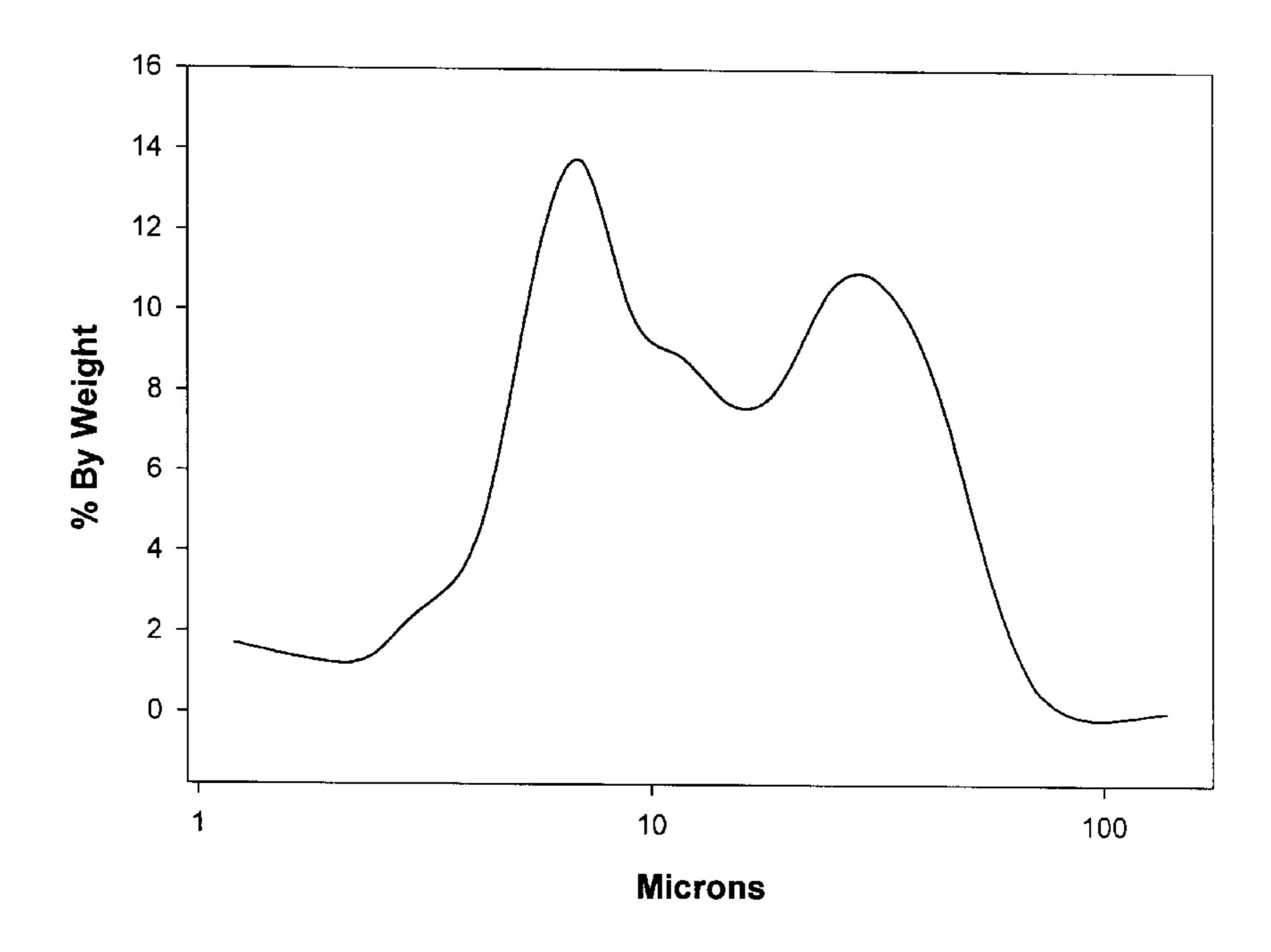
Figure 1 Bi-modal particle size distribution of water insoluble solids in conventional peanut butter
