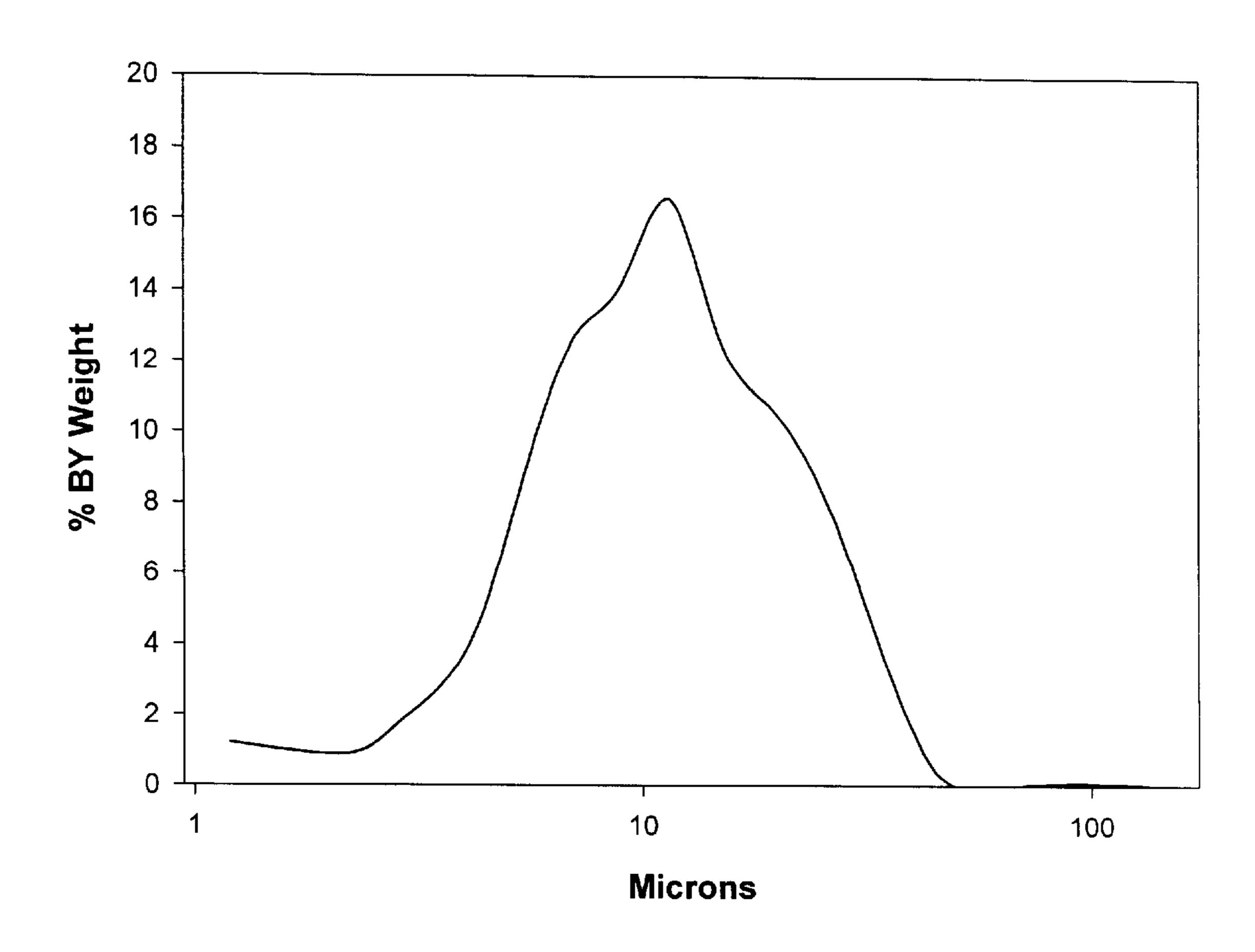
Figure 4a Mono-modal particle size distribution of product made according to the present inventioon
