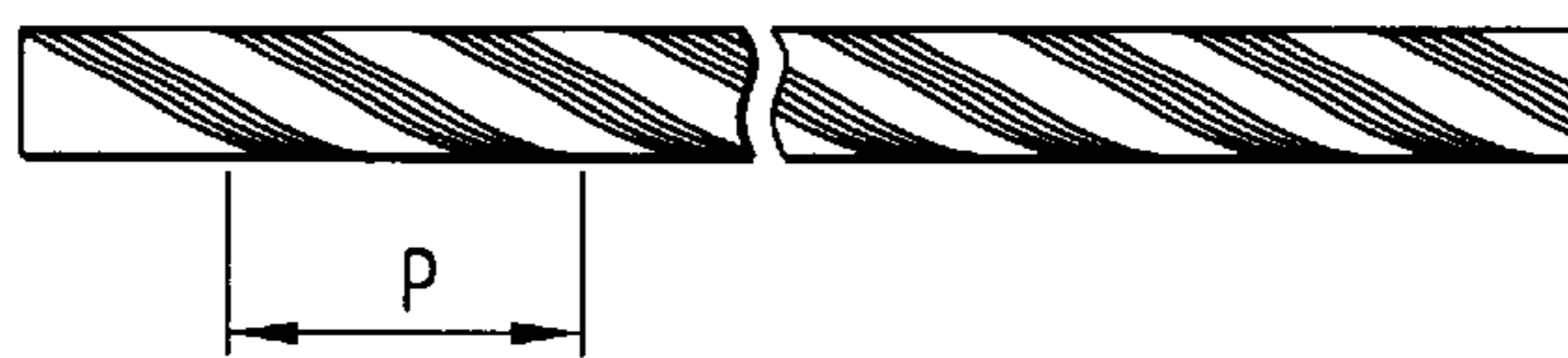
A EXAMPLE OF A PARALLEL CONDUCTOR
