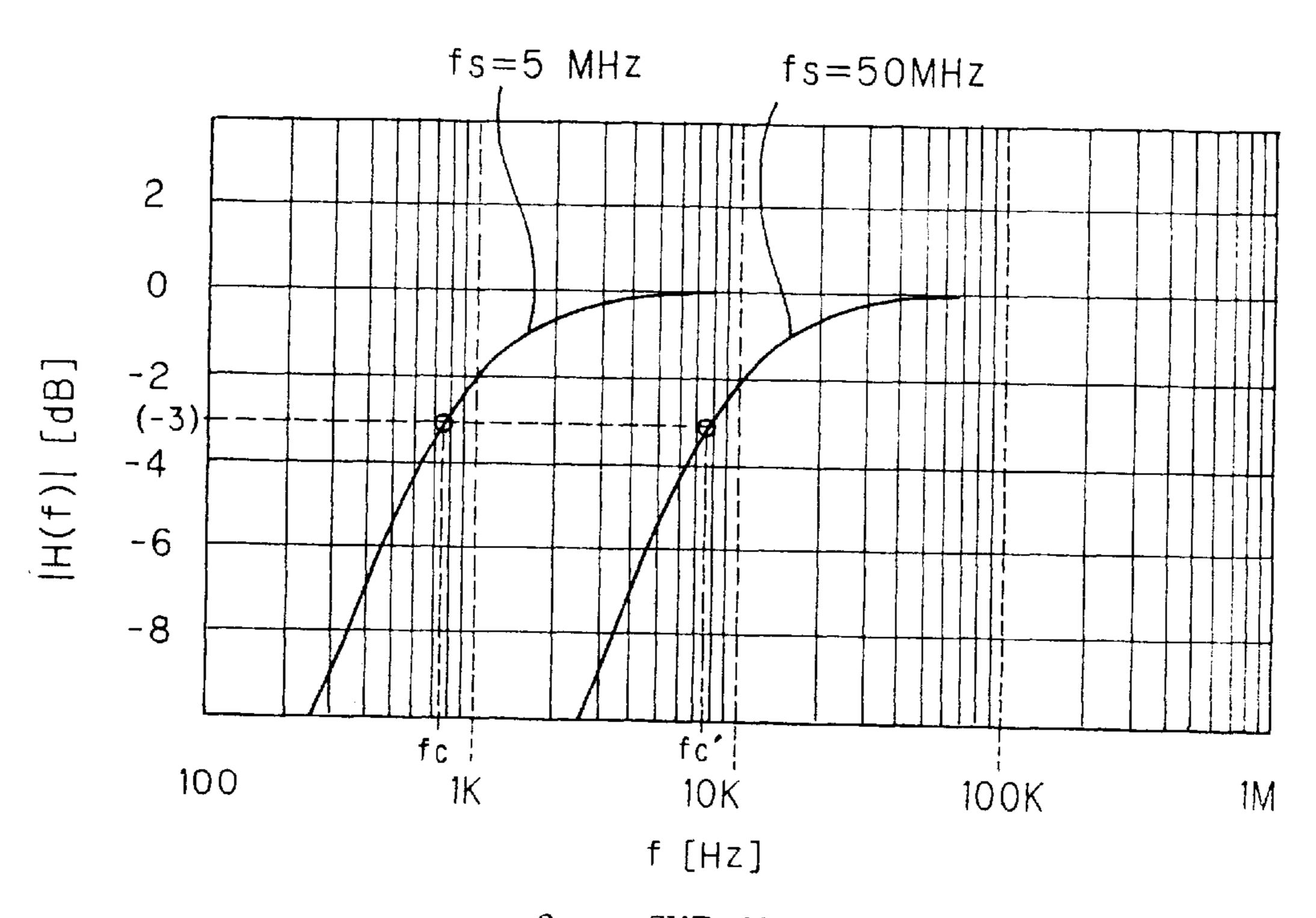
fc: CUT-OFF FREQUENCY WHEN fs=5MHz fc': CUT-OFF FREQUENCY WHEN fs=50MHz
