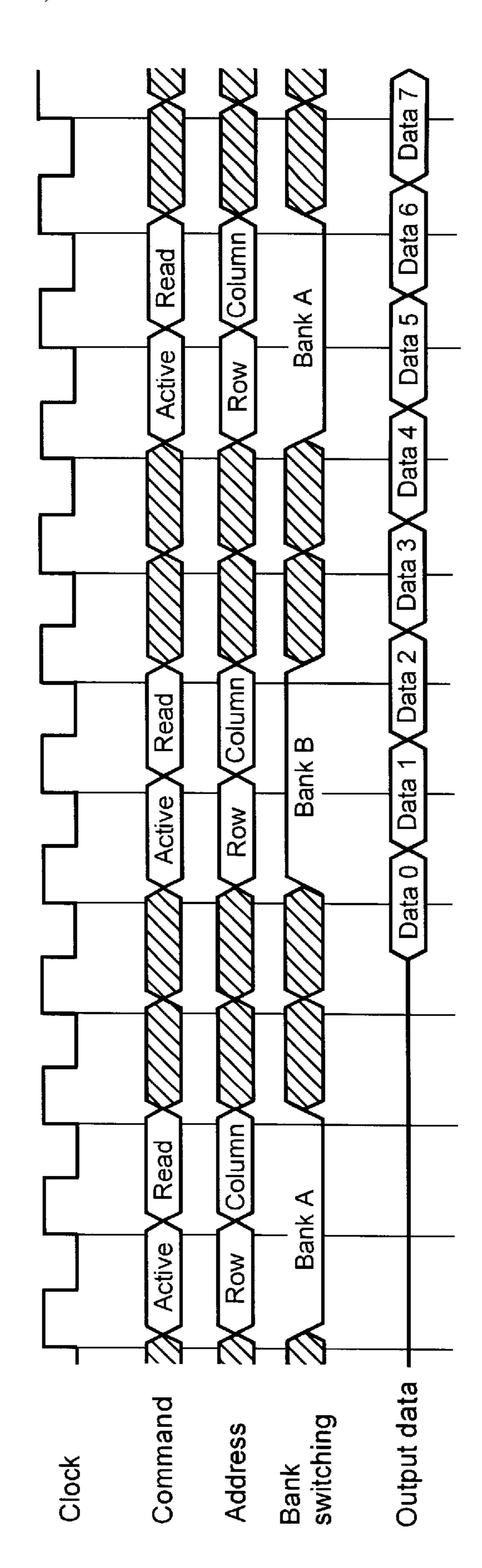
SDRAM operation transfer timing chart by bank switching
