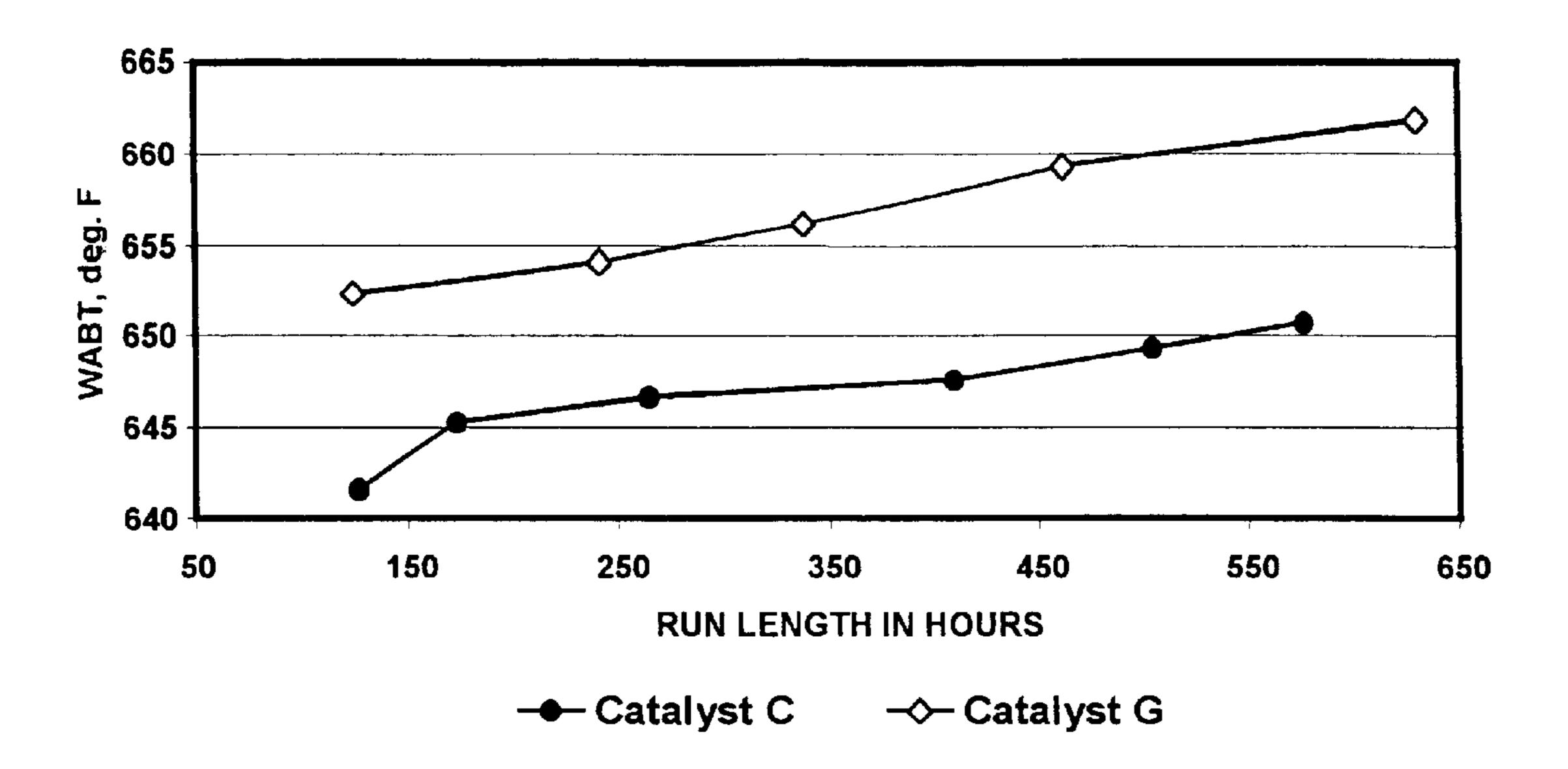
FIGURE 4. WABT REQUIRED FOR 30% BASIC NITROGEN REMOVAL
