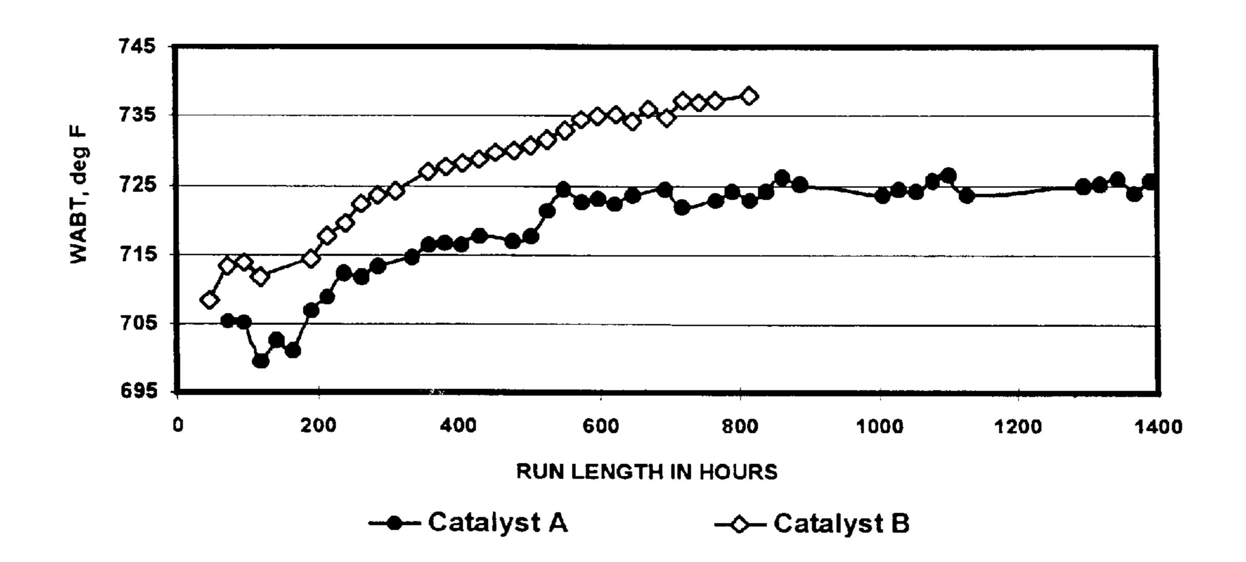
FIGURE 2. WABT REQUIRED FOR 88% SULFUR REMOVAL
