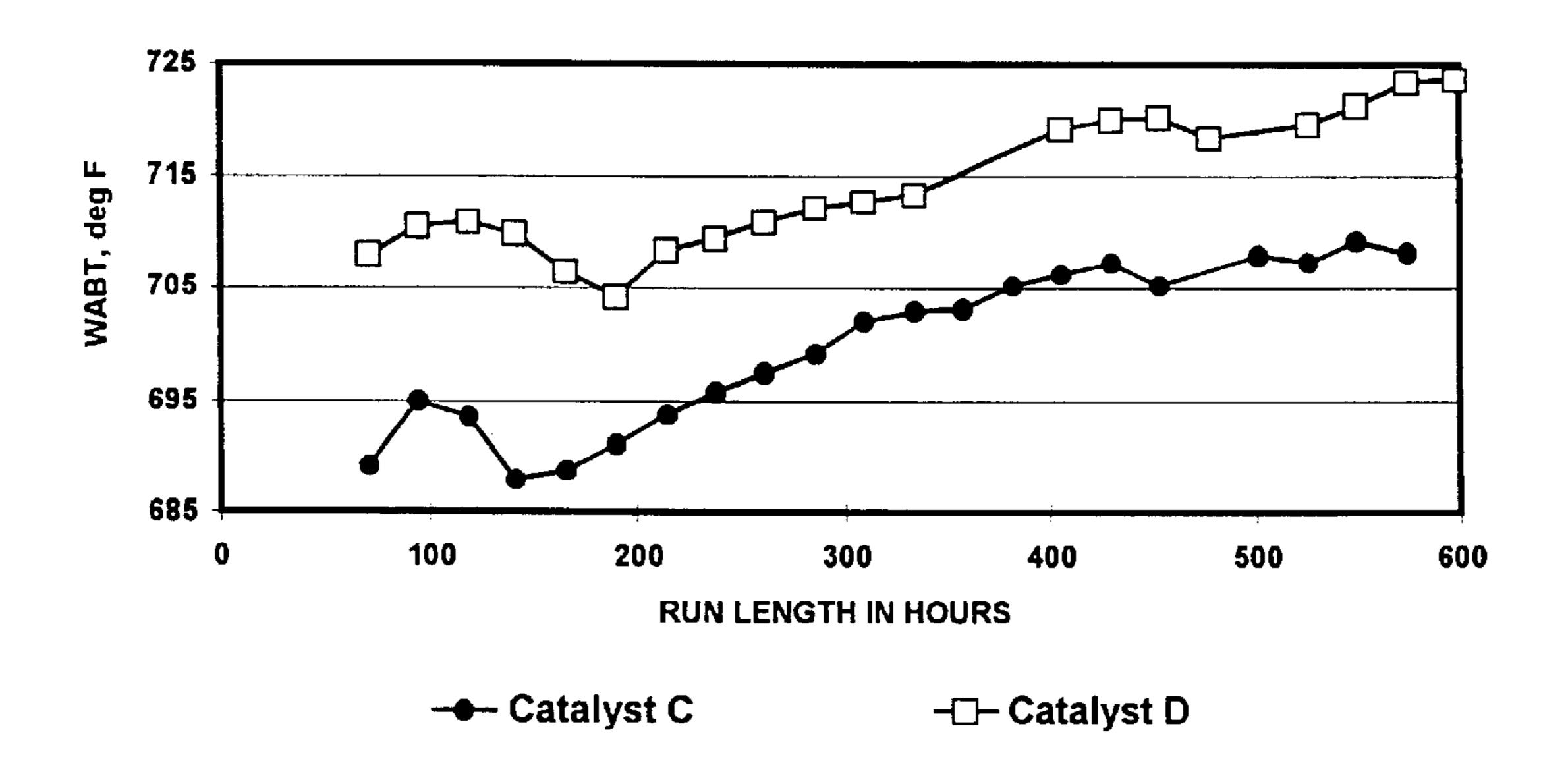
FIGURE 3. WABT REQUIRED FOR 30% TOTAL NITROGEN REMOVAL
