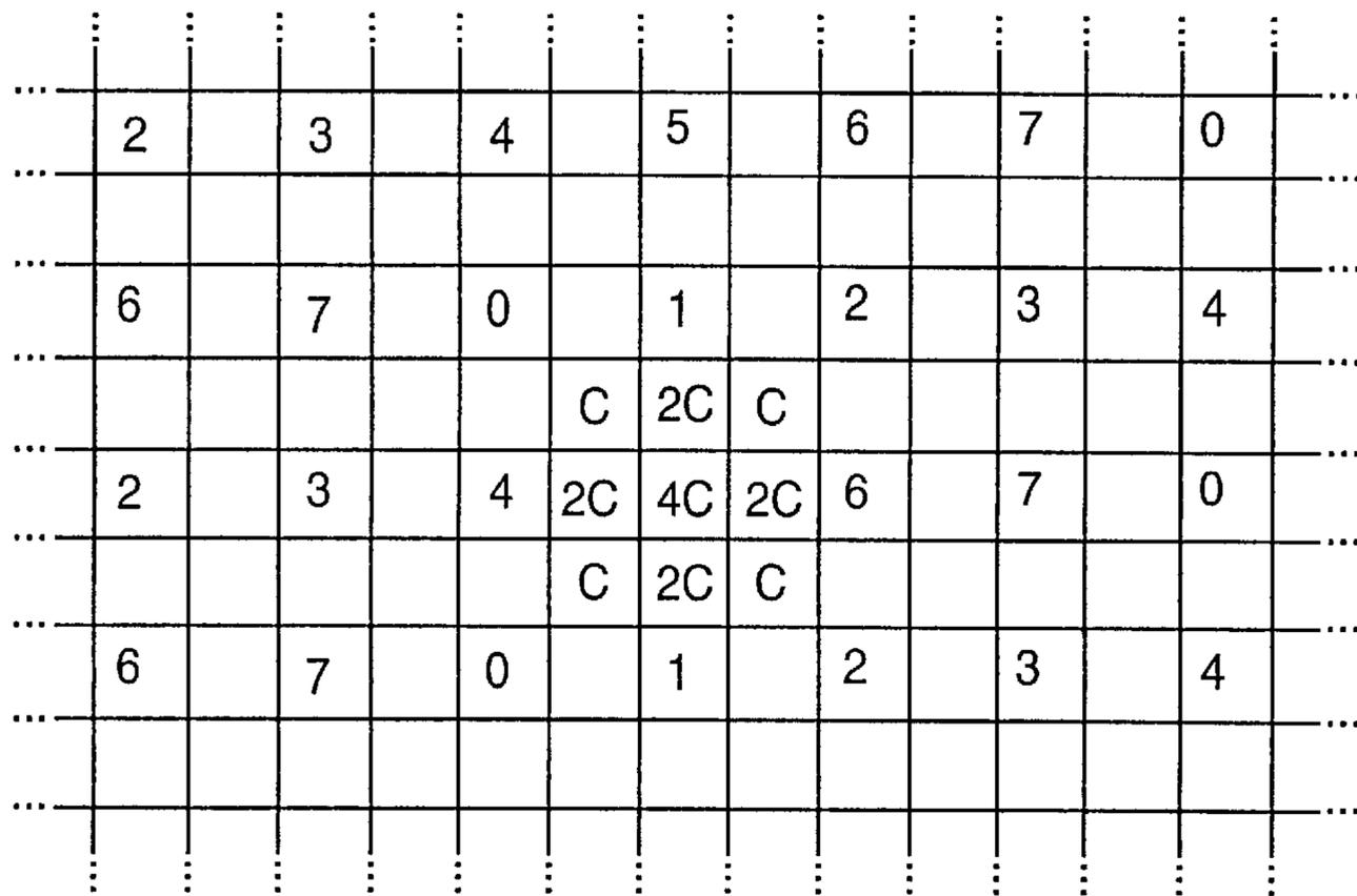
EXAMPLE OF HOW MANY ELEMENTARY BUMPS, 900, WOULD BE ASSIGNED LOCATIONS IN AN IMAGE, AND THOSE LOCATIONS WOULD BE ASSOCIATED WITH A CORRESPONDING BIT PLANE IN THE N-BIT WORD, HERE TAKEN AS N=8 WITH INDEXES OF 0-7. ONE LOCATION, ASSOCIATED WITH BIT PLANE "5", HAS THE OVERLAY OF THE BUMP PROFILE DEPICTED.
