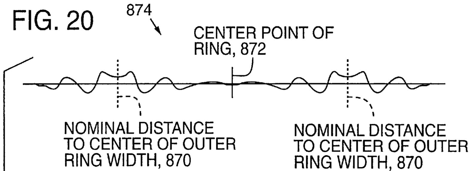
2-D BRIGHTNESS OF PHASE-ONLY FILTERED RING IS SIMILAR TO THE ABOVE BRIGHTNESS PATTERN ROTATED ABOUT CENTRAL POINT OF RING:
