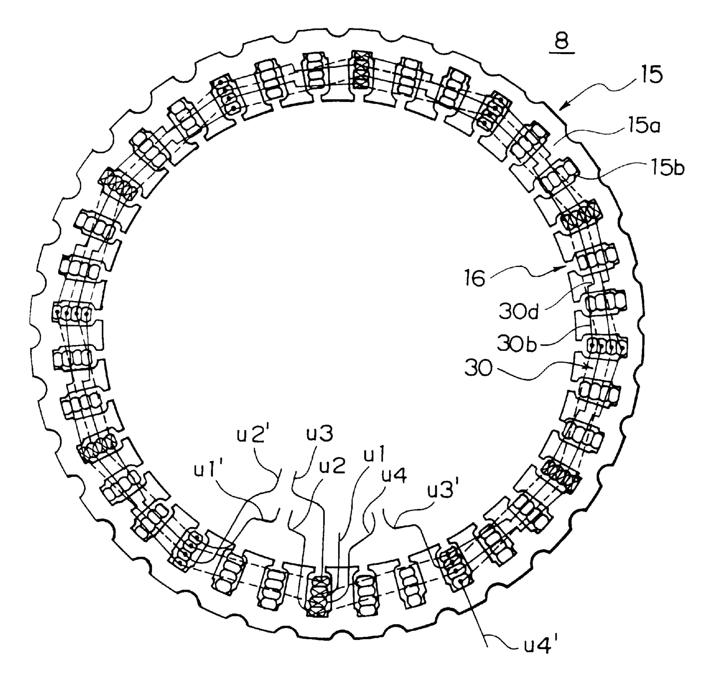
SOLID LINES: WIRES AT NON-CONNECTION SIDE (REAR SIDE)
