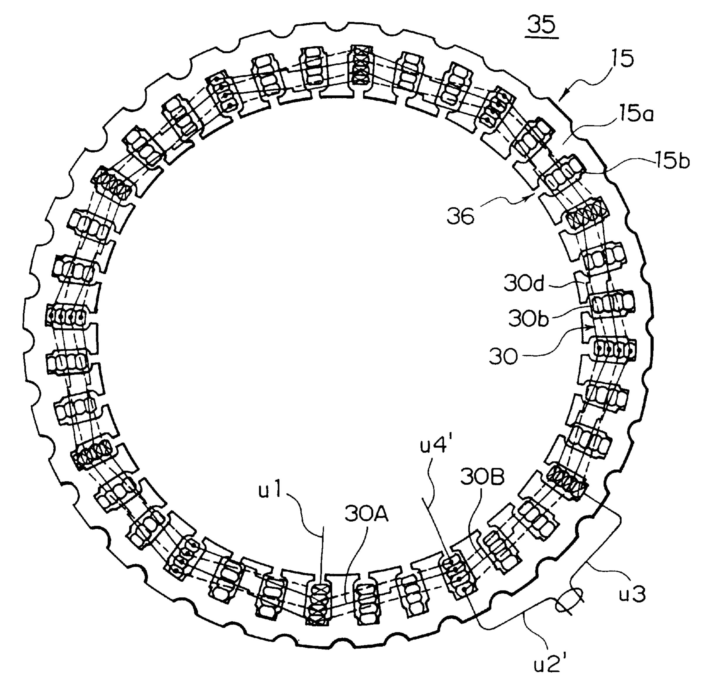
SOLID LINES: WIRES AT NON-CONNECTION SIDE (REAR SIDE) DOTTED LINES: WIRES AT CONNECTION SIDE (FRONT SIDE)
