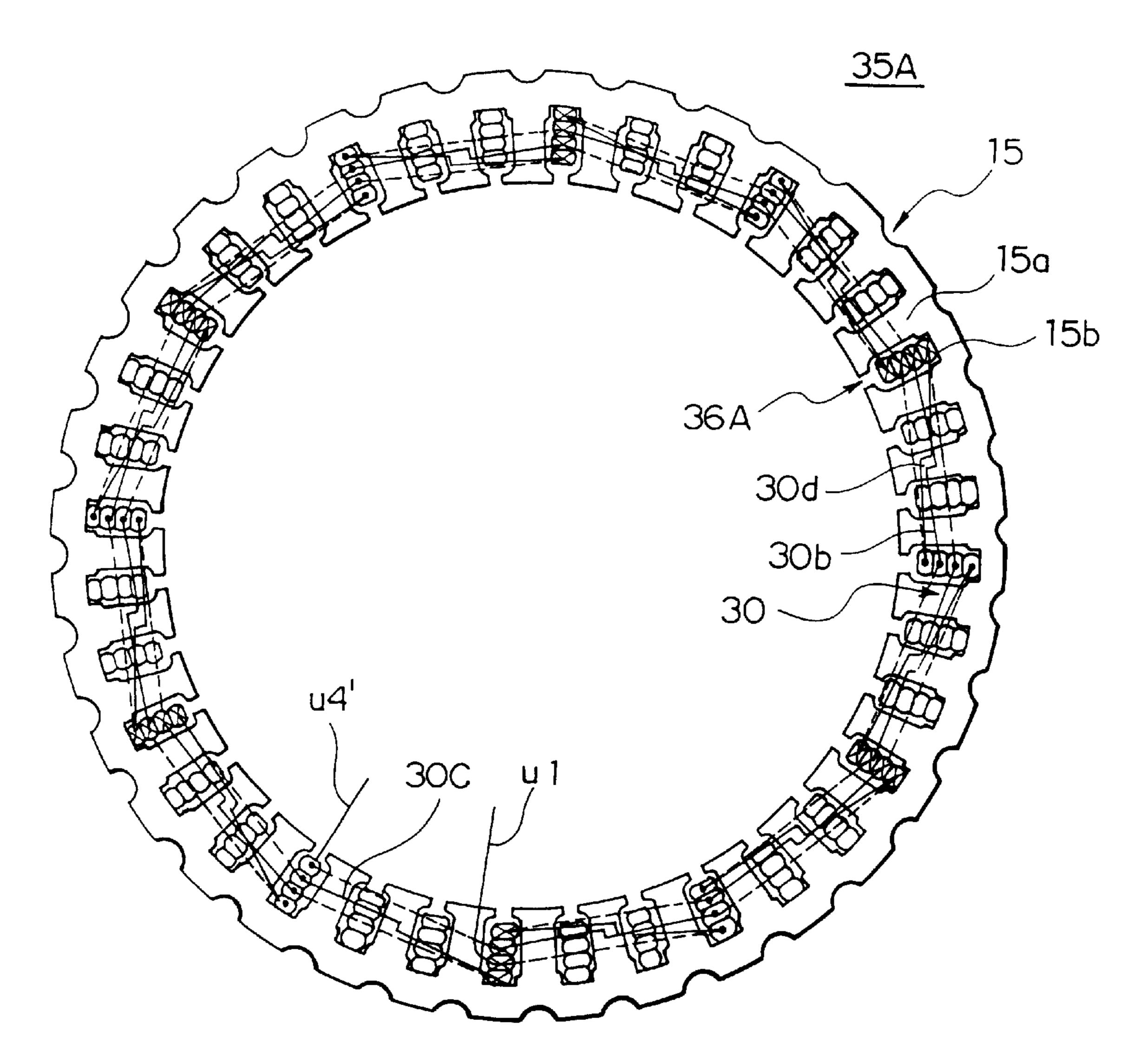
SOLID LINES: WIRES AT NON-CONNECTION SIDE (REAR SIDE) DOTTED LINES: WIRES AT CONNECTION SIDE (FRONT SIDE)
