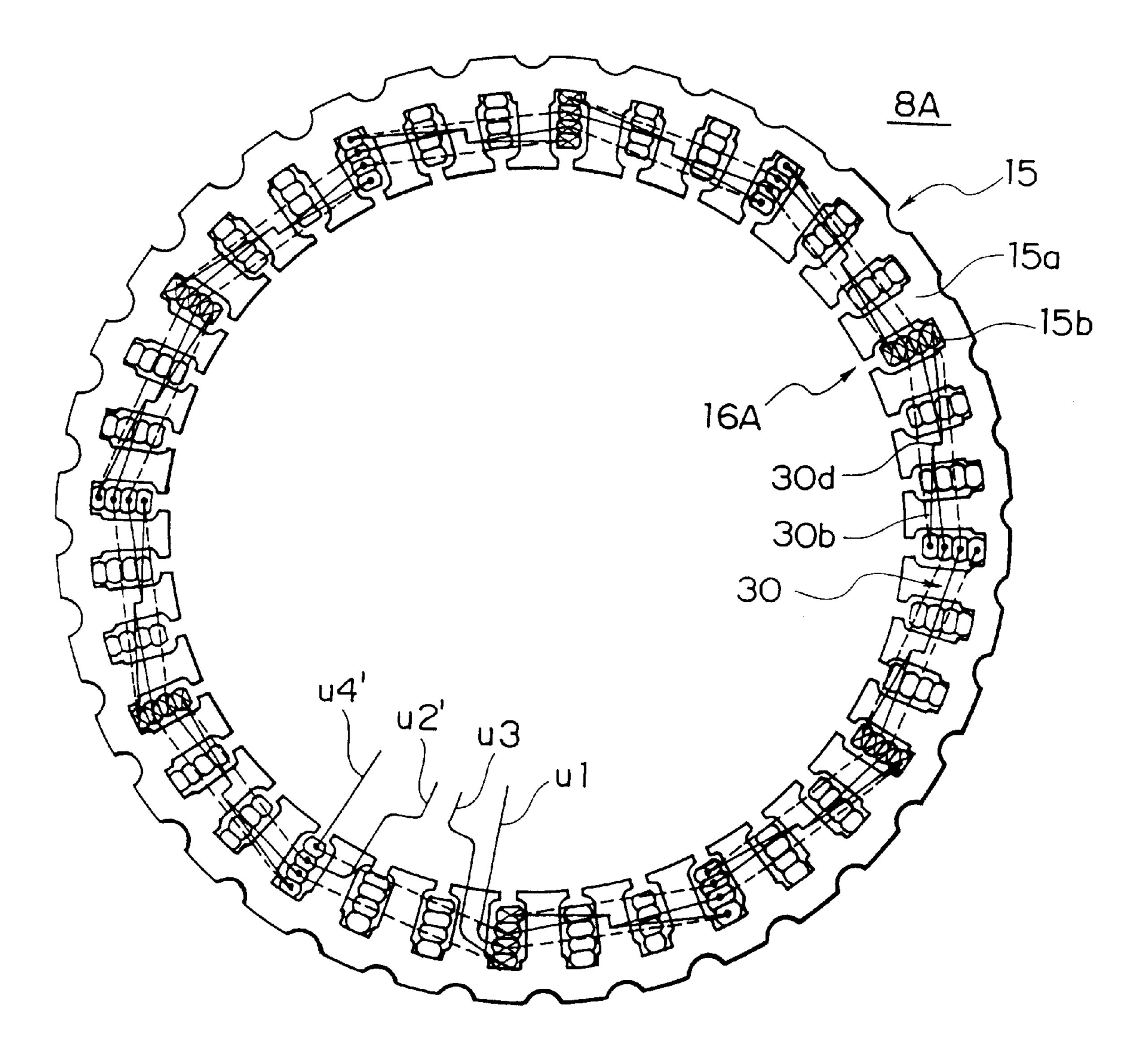
SOLID LINES: WIRES AT NON-CONNECTION SIDE (REAR SIDE)
