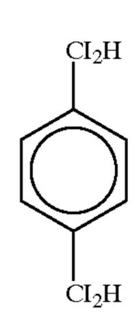
$\alpha$ ,  $\alpha$ ,  $\alpha$ ',  $\alpha$ '-tetrachloro-p-xylene (hereinafter "TCPX") having the molecular structure:
