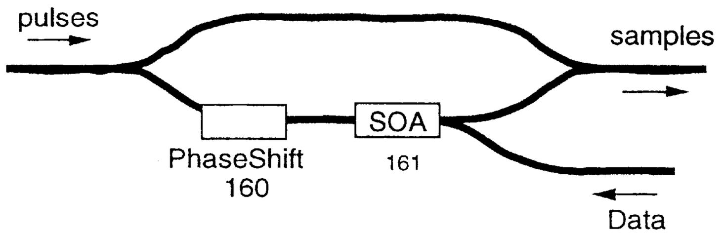
Fig 21 Two stage interferometer arrangement
