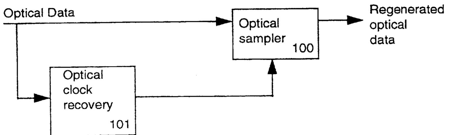
Fig 12 Optical Regenerator
