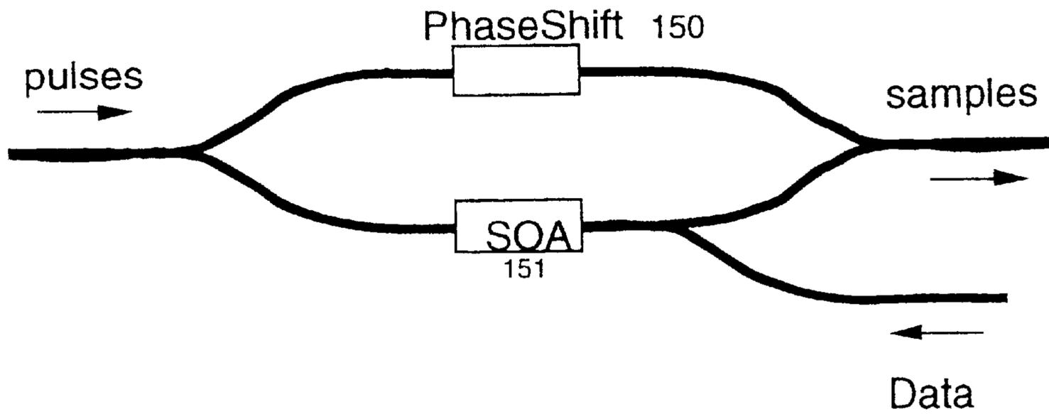
Fig 20 Interferometer Arrangement
